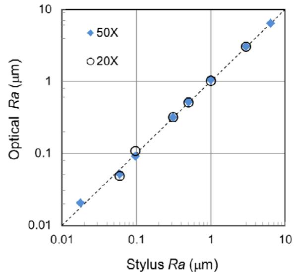
FIGURE 6. Graphical representation of the results on Rubert sinusoidal roughness specimens at 20X and 50X magnifications. The diagonal line represents perfect correlation.
