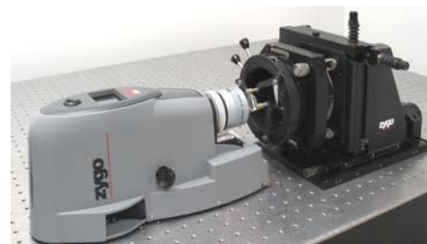
PTI in horizontal arrangement with 3-Axis Mount, Tip/Tilt Mount, and Self Centering Element Holder
