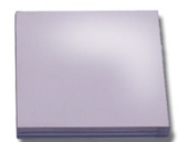
Step Height Standards used to verify vertical accuracy 0.088 \mu\text{m} step, (p/n 1776-666-009) 1.75 \mu\text{m} step, p/n 1776- 666-010 24.0 \mu\text{m} step, (p/n 1776-666-011)
