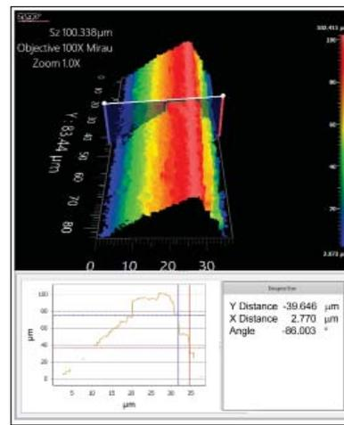
**Figure 4: Commercial razor blade measured on edge shows a measurable surface slope of 86°.**
