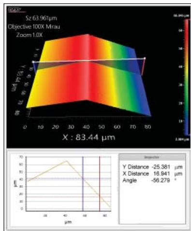
**Figure 3: Quartz rod tilted 10° to present one surface at 56°.**
