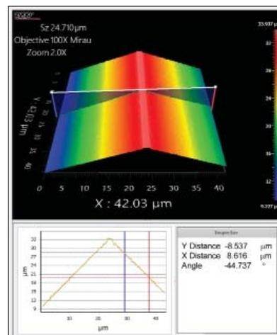
Figure 2: 45° slope measured on the Nexview™.
