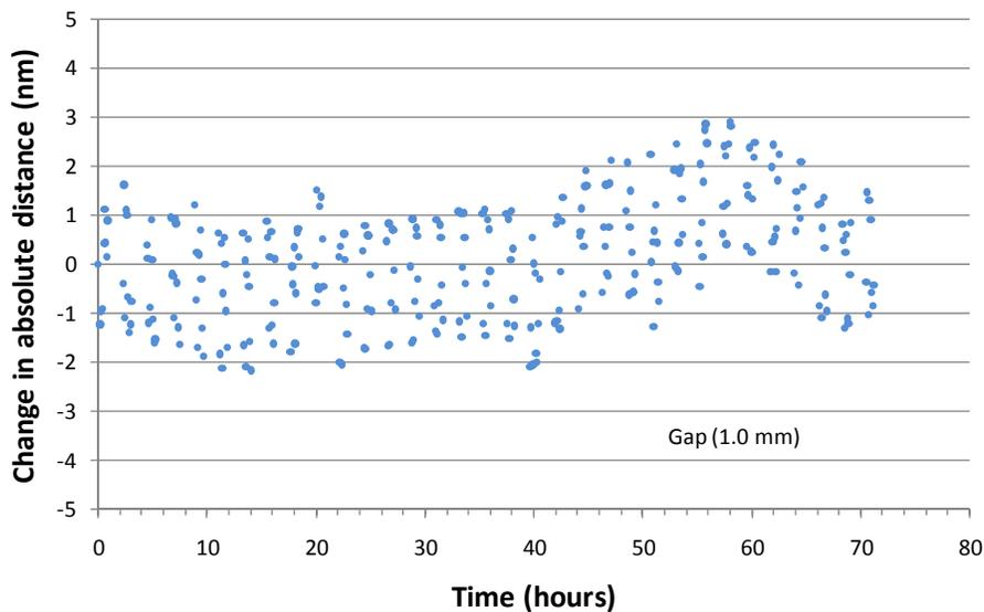
Figure 8: A plot of 300 measurements over 72 hours of the absolutely known cavity using the ADMI.
