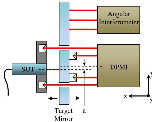
Figure 6: Setup used to compare the ADMI relative and absolute measurement modes against simultaneous measurements of a ZMI-4000 for a 500 $\mu$ m scan centered about the beam waist.
