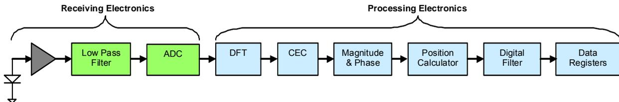
Figure 5: Channel amplification, digitization and phase computation flow.
