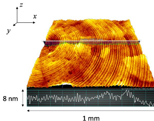
**Figure 1.** An example of optical surface topography measurement requiring nm-level sensitivity to surface heights.
