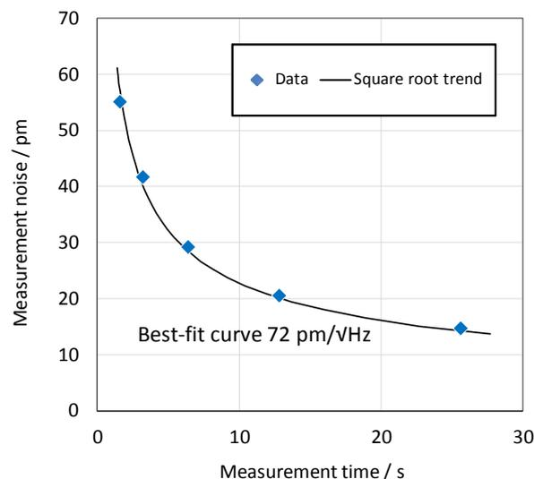
**Figure 2.** Experimental demonstration of the reduction of measurement noise as a function of data acquisition time for the ZYGO Nexview™ 3D interference microscope.
