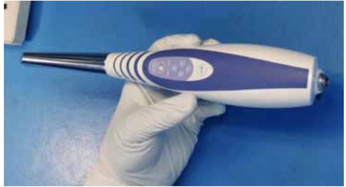
*With a knowledgeable partner, optical subassemblies, or even final assemblies like this 3D dental imaging wand, including 20 optics and 3 imaging sensors in an autoclave compatible case, can be custom manufactured for you.*
