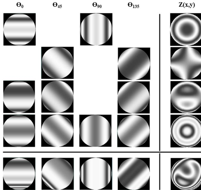
Figure 2. Recreation of Zernike polynomials from angular decomposition ( $0^\circ, 45^\circ, 90^\circ, 135^\circ$ )
