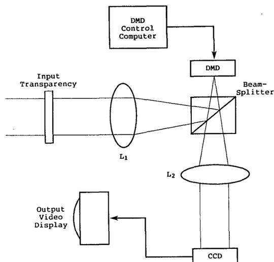
Fig. 1. Diagram of the DMD correlator system.
