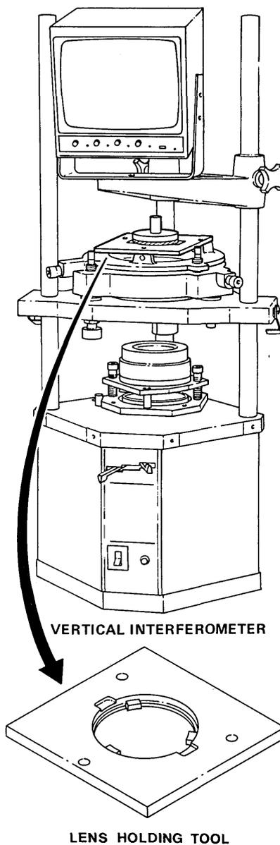
Fig. 1. Vertical interferometer and lens holding tool.
