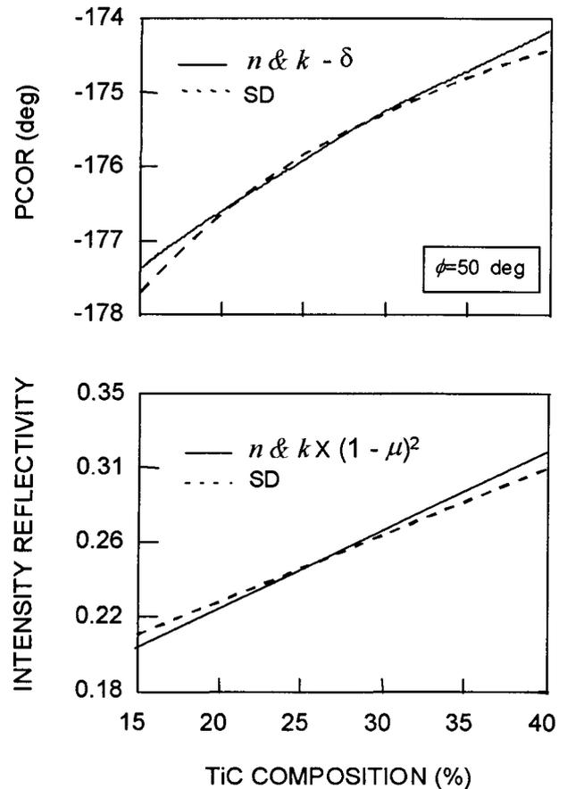
Fig. 8. Theoretical s-polarization PCOR and intensity reflectivity with the constant  $\mu = 9.5\%$  and  $\delta = 3.8^\circ$  offsets, as a function of the TiC composition  $\epsilon$  at an incident angle of 50°. The  $\mu$  and  $\delta$  make it possible to continue to use  $n$  and  $k$  to map changes in Al<sub>2</sub>O<sub>3</sub>-TiC composition.
