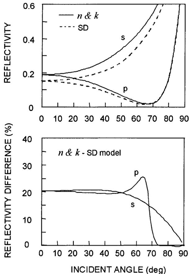
Fig. 6. Comparison of the predicted intensity reflectivities  $R$  for the  $n$ -and- $k$  model and  $R$  for the SD model. The SD model predicts a 20% relative intensity difference at normal incidence, confirming the experimental results in Table 1.
