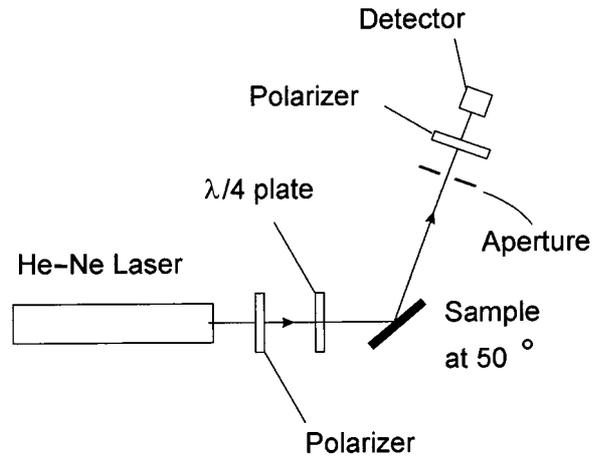
Fig. 2. Null ellipsometer using a 633-nm He-Ne laser.
