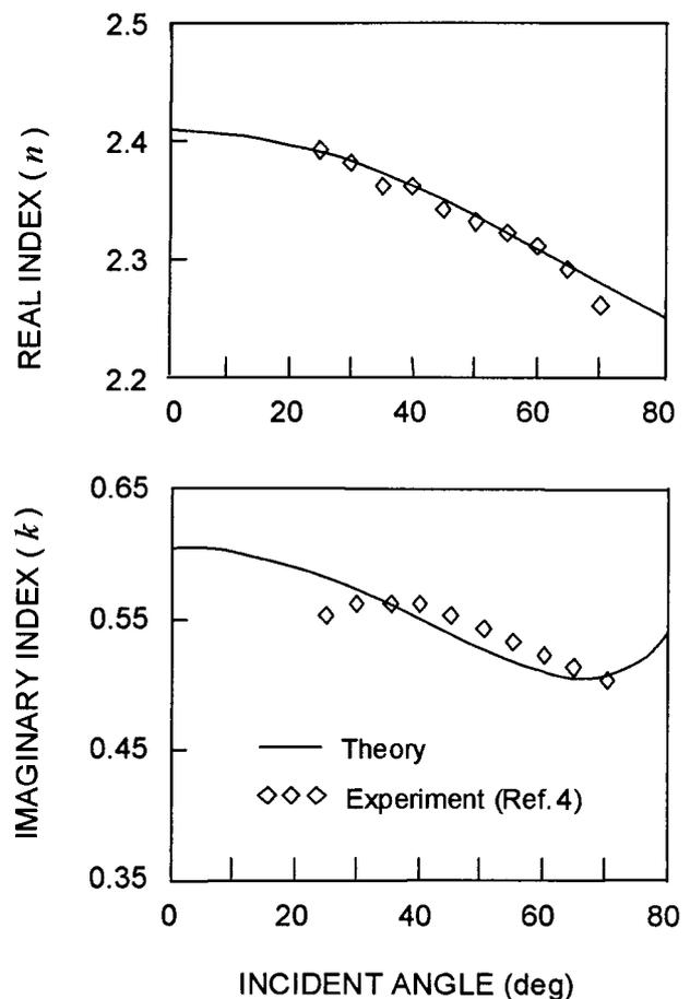
Fig. 5. Comparison of experimental and theoretical variation of measured  $n$  and  $k$  with incident angle for  $\text{Al}_2\text{O}_3$ -TiC. The experimental data are from Ref. 4. For a true homogeneous material,  $n$  and  $k$  would be constant.
