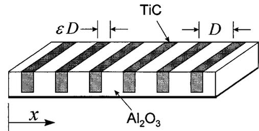
Fig. 3. Simple model of composite  $\text{Al}_2\text{O}_3$ -TiC that comprises stripes of TiC embedded in  $\text{Al}_2\text{O}_3$ .
