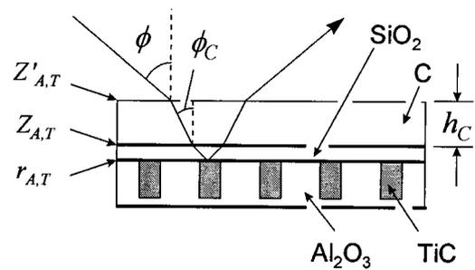
Fig. 10. Simple model of  $\text{Al}_2\text{O}_3$ -TiC with a DLC coating and a  $\text{SiO}_2$  adhesion layer.
