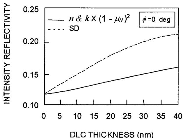
Fig. 12. Intensity reflectivity at normal incidence for variable DLC thickness for a nominal scatter-loss coefficient  $\mu_N = 10\%$ . The ellipsometry for  $n$  and  $k$  is calculated at a  $50^\circ$  incident angle, and the TiC composition is  $\epsilon = 20\%$ . The large divergence forces a reduction of the  $\mu_N$  factor from 10% to a compromise value of 5%.
