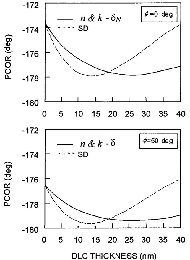
Fig. 11. PCOR at normal incidence and at an incident angle  $\phi$  of  $50^\circ$  for the  $n$ -and- $k$  and the SD models, for variable DLC thickness. For a fixed relative TiC composition,  $\epsilon = 20\%$ . The ellipsometry for  $n$  and  $k$  in both cases is calculated at  $50^\circ$ . The  $n$ -and- $k$  model prediction includes the offsets  $\delta = -3.8^\circ$  and  $\delta_N = -4.2^\circ$ .
