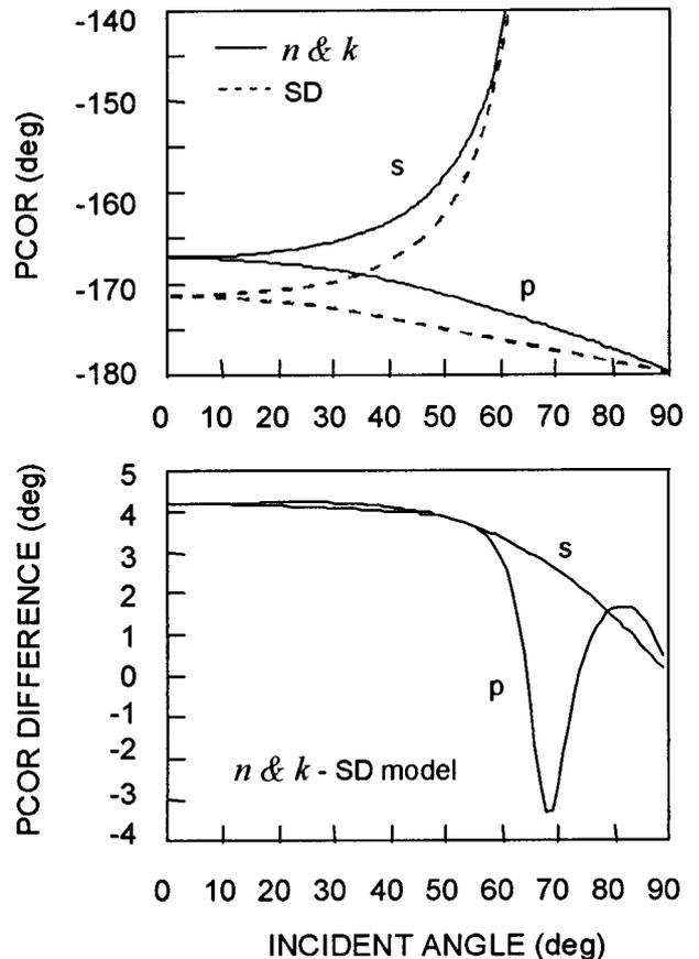
Fig. 7. Theoretical PCOR. The SD model predicts a PCOR at normal incidence that is  $4^\circ$  lower than the value calculated with the effective  $n$  and  $k$ .
