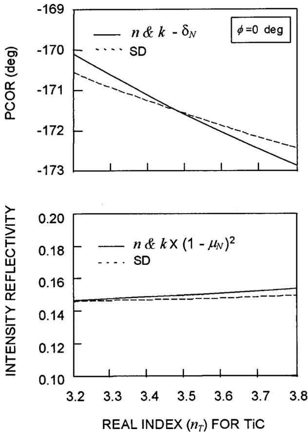
Fig. 9. Theoretical s-polarization PCOR and intensity reflectivity at normal incidence as a function of a variable refractive index for TiC. The  $n$  and  $k$  results include the constant offsets  $\mu_N = 10\%$  and  $\delta_N = 4.2^\circ$ . The TiC composition  $\epsilon$  is fixed at 30%.
