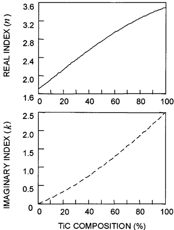
Fig. 4. Predicted effective  $n$  and  $k$  values as a function of the TiC composition  $\epsilon$ , according to the SD model in the low-N.A. limit.
