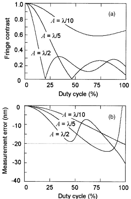
Fig. 4. (a) Dependence on duty cycle  $D$  of the fringe contrast at a vibrational phase of  $\varphi_0 = 0$ . (b) Dependence on  $D$  of the relative measurement error (which equals the error divided by the vibrational amplitude  $\Lambda$ ) at a vibrational phase of  $\varphi_0 = \pi/2$ .
