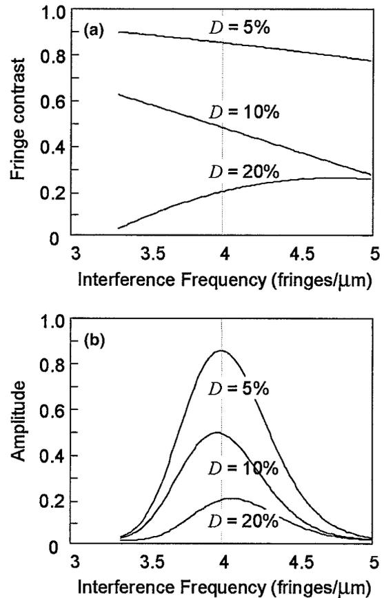
Fig. 2. (a) Dependence of the fringe contrast on interference spatial frequency. (b) Resultant distortion in the frequency domain of an interferometer signal, showing, in particular, a shift in the peak wavelength. Vibrational amplitude of 250 nm, vibrational phase of 0, and three different pulse duty cycles.
