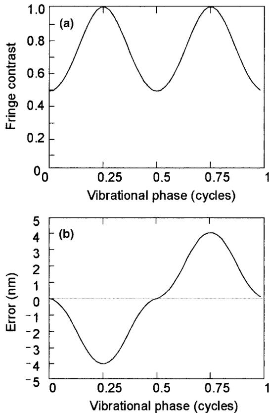
Fig. 1. (a) Variation in fringe contrast with vibrational phase  $\varphi$ . (b) Variation in measurement error with vibrational phase  $\varphi$ . Duty cycle of  $D = 10\%$ , vibrational amplitude of  $\Lambda = 250$  nm.
