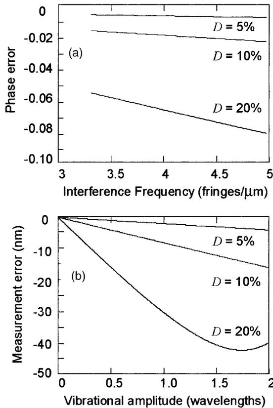
Fig. 3. (a) Dependence on interference spatial frequency  $K$  of the phase error (argument of  $u$ ) attributable to stroboscopic interferometry for a vibrational amplitude of  $\Lambda = 250$  nm and a vibrational phase of  $\varphi_0 = \pi/2$ . (b) Resultant measurement error as a function of vibrational amplitude.
