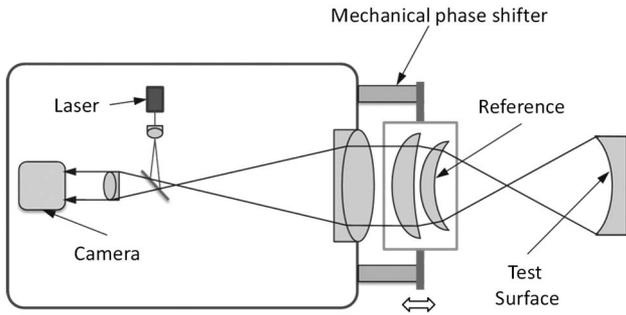
Fig. 2. Laser Fizeau interferometer with a spherical cavity.
