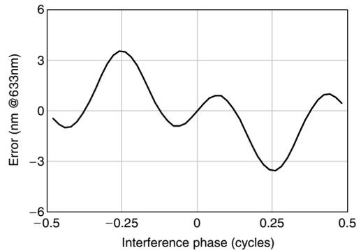
Fig. 6. Phase-dependent measurement errors for the three-frame algorithm in the presence of  $-20\%$  detuning in a  $4\%$ – $4\%$  Fizeau cavity.
