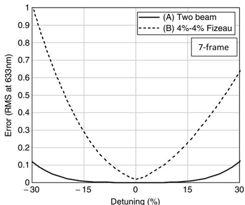
Fig. 1. Sensitivity of a high-performance seven-frame PSI algorithm [7] to phase-shift calibration errors, assuming (A) two-beam interference, as is the usual approach to error analysis, and (B) interference in a laser Fizeau cavity with modest 4% reference and 4% object reflectivities.
