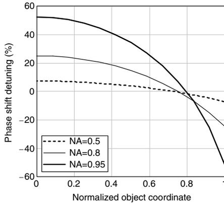
Fig. 4. Phase shift calibration error as a function of the normalized field coordinate in a spherical Fizeau cavity for three different cavity NA values.
