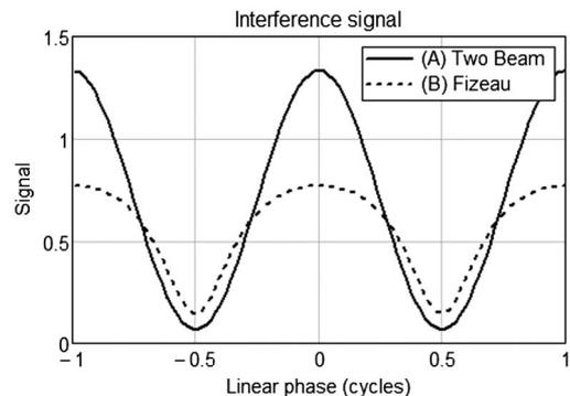
Fig. 3. (A) Interference fringe signal for a linear phase shift in a two-beam interferometer such as a Michelson, Twyman Green, or low-coherence microscope. (B) Interference signal for a laser Fizeau interferometer with reference and object reflectivities, both of which equal 20%.
