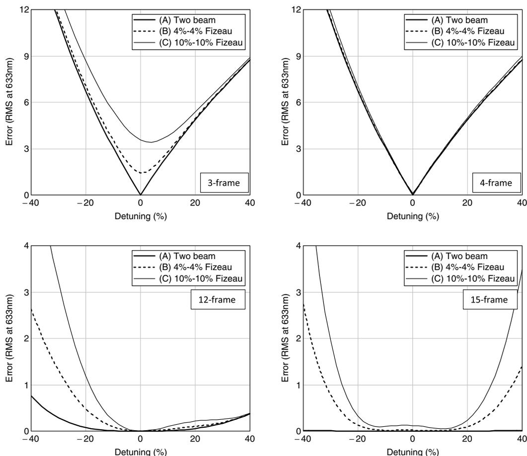
Fig. 7. Sensitivity of PSI algorithms to calibration errors for three different interferometer configurations: (A) Two-beam interferometer. (B) Fizeau interferometer with 4% reflectivity for both surfaces. (C) Fizeau interferometer with 10% reflectivity for both surfaces. Note the 3 $\times$  change in scale between the upper two graphs and the lower two graphs in the figure.
