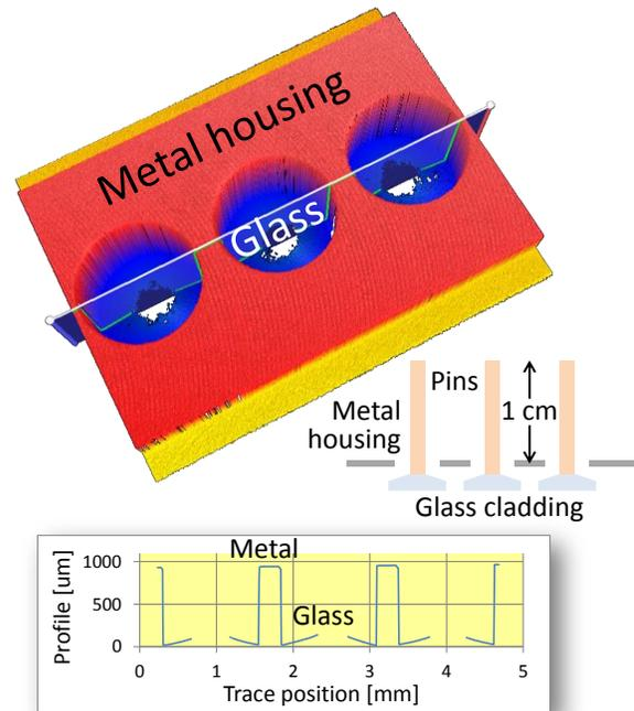
FIGURE 7. Electrical feed-through assembly. Of primary interest is the glass cladding, recessed below the metal housing along with pins extending  $\sim 1$  cm beyond the housing. Blue regions in the height map correspond to glass, with missing data indicating the location of pins.
