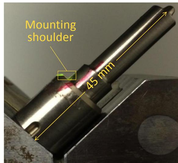
FIGURE 5. Photograph of fuel injector, with mounting shoulder region outlined in yellow.
