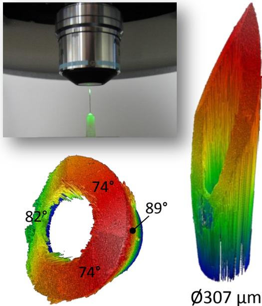
*FIGURE 8. Hypodermic needle measured end-on in a single FOV. Upper left: photograph of setup. Right: obtained data over 1.8-mm scan range. Lower left: same data rotated to show measured slopes up to 89° and automatic identification of bore region.*
