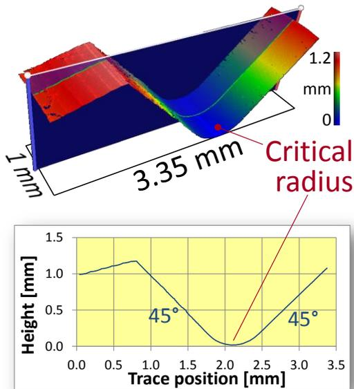
FIGURE 6. Measurement of shoulder region of fuel injector, highlighting radius critical for proper sealing with engine block.
