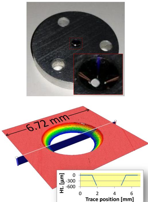
FIGURE 2. Measurement of 5-mm-diameter diamond-turned  $90^\circ$  cone in a single FOV. Top: photograph of part; bottom: measured height map.
