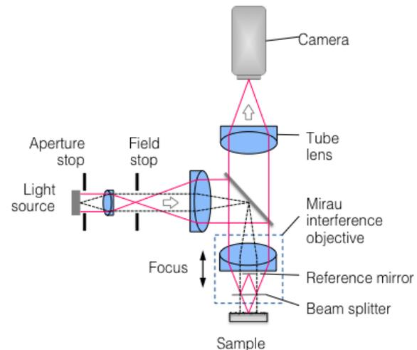
FIGURE 1. Schematic representation of Coherence Scanning Interferometry.
