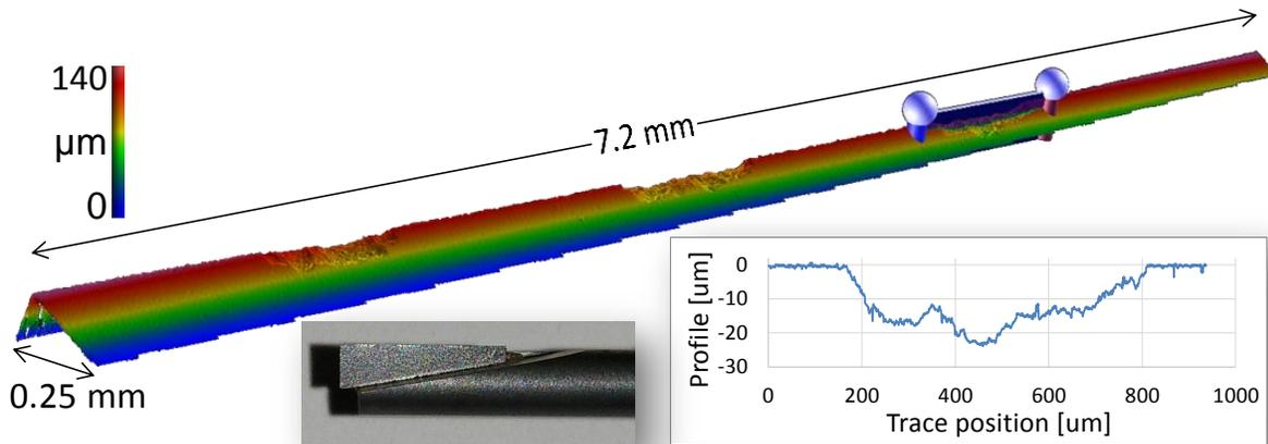
FIGURE 4. End-mill measured with  $0.4\ \mu\text{m}$  lateral sampling over 7.2-mm length and  $145\text{-}\mu\text{m}$  scan range in about 9 minutes. Photograph of part is shown in lower left inset.
