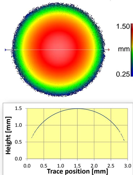
FIGURE 3. 3-mm-diameter sealing ball measured in a single FOV for local slopes up to  $60^\circ$ .
