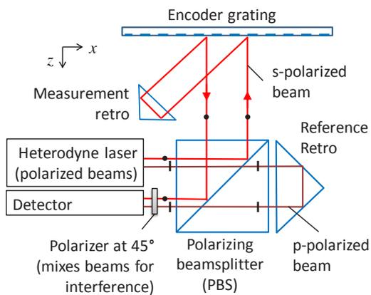
FIGURE 1: Basic encoder geometry using a linear interferometer.
