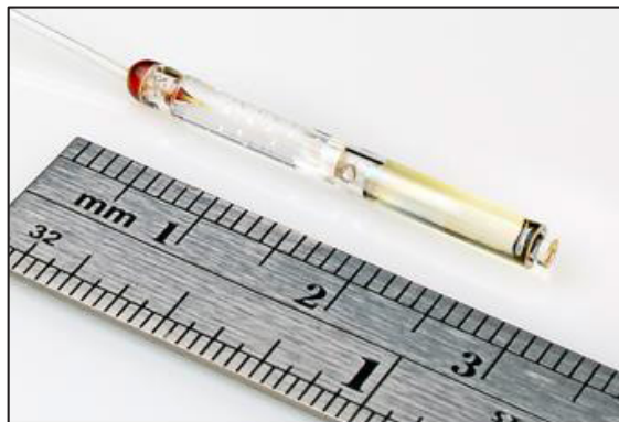
FIGURE 6: High-precision, fiber-based position sensing system [13, 14].
