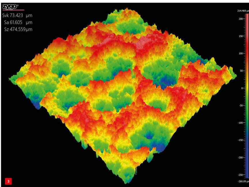
Measurements of the dark, rough features after the TBC application can provide process engineers information on the formation and distribution of surface porosity. The height scale runs from  $-260$  to  $+214$   $\mu\text{m}$ , the XY dimensions are approx.  $1$   $\text{mm} \times 1$   $\text{mm}$ .
