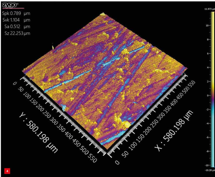
honed surfaces displays the full dynamic range of the Zygo CSI-based optical profiler systems. The development of specialised hardware and software enhancements has significantly improved this capability, enabling measurements of previously inaccessible steep surfaces and super-polished surfaces with one metrology solution.
