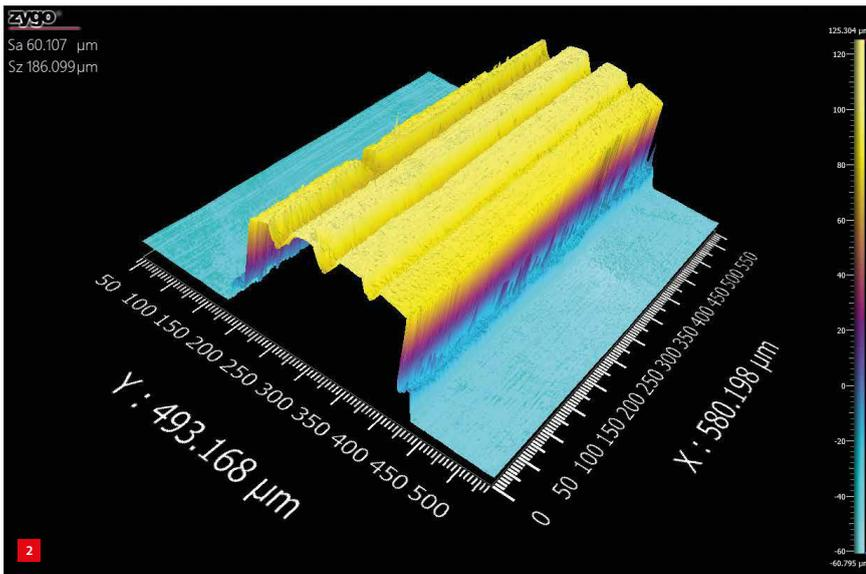
CSI scan of the mechanically activated surface that will provide the anchor for the thermal barrier coating to adhere to the cylinder wall surface. The height scale runs from  $-66$  to  $+125$   $\mu\text{m}$ .
