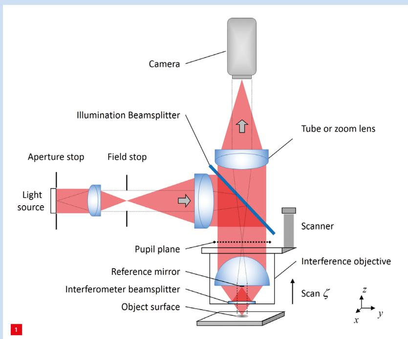
1 Typical set-up for coherence scanning interferometry; see the text for explanation.
