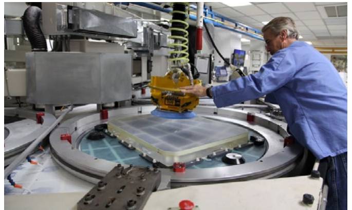
Refurbishing highly durable coated optics requires in-house grinding and polishing capabilities.
