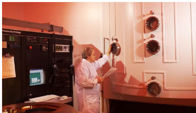
High reflective, antireflective and specialty coatings are applied in 72-inch coating chambers.
