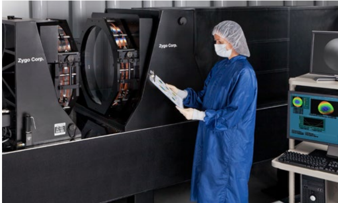
Large aperture interferometry ensures optics meet specifications before and after coating.
