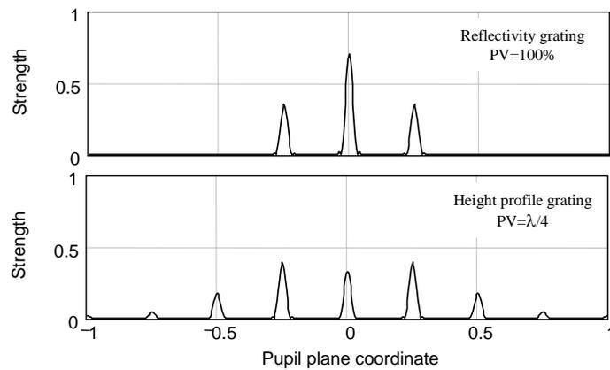
**Figure 2:** Comparison of the diffracted beams from *amplitude* (upper) and *phase* (lower) gratings illustrates the complex diffraction behavior of height objects, leading to nonlinear response when profiling surface heights.
