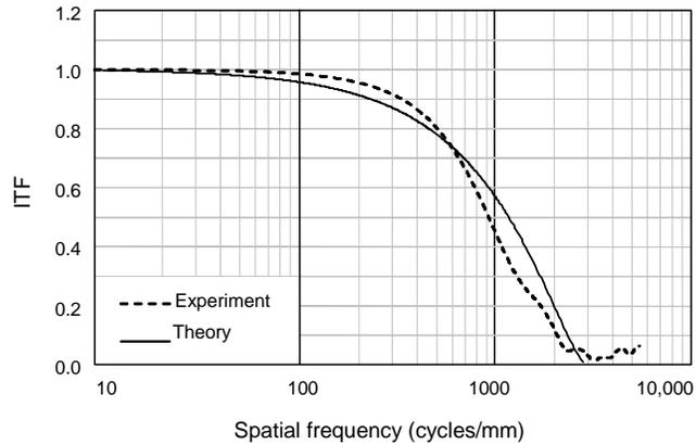
**Figure 3:** Comparison of the theoretical ITF magnitude (Eq.(4)) and experimental results for a white-light interference microscope using a 100X, 0.8 NA Mirau objective and incoherent illumination. The data derive from the profile of a 40-nm step object.
