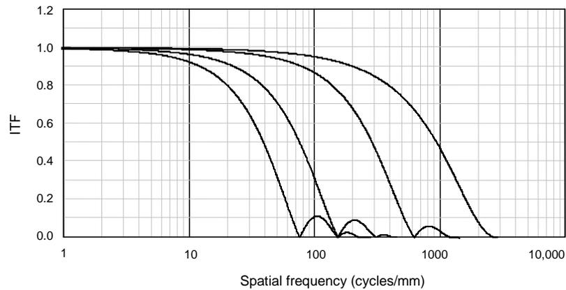
**Figure 5:** Theoretical ITF curves for 2.5X, 5X, 20X and 100X microscope objectives illustrate the spatial frequency overlap achieved in typical microscopes setups, and the influence of the camera at low magnification.
