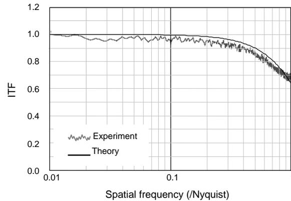
**Figure 4:** The predicted and experimental ITF curves for this 100-mm aperture coherent laser Fizeau interferometer are dominated by the lateral resolution of the 640X480 camera. Here the data stop at Nyquist because the sampling is too sparse above this frequency.
