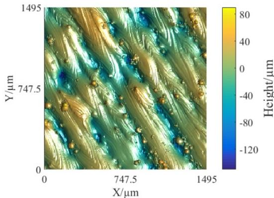
FIGURE 1: Surface manufactured using a laser powder bed fusion process, illustrating the mix of deterministic and random structures, measured with a focus variation microscope
