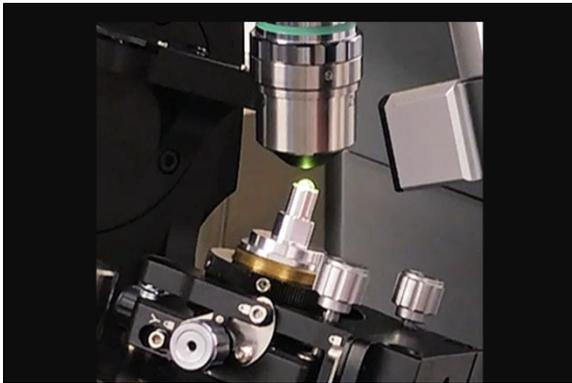
FIGURE 2: Micro-asphere metrology using high-slope measurements at multiple viewing angles in an interference microscopy.
