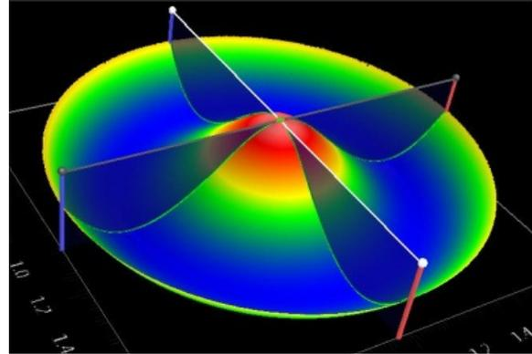
FIGURE 3: Example measurement of a 1.8 mm diameter microlens having 60  $\mu\text{m}$  of aspheric departure. Cross-sections are indicated for illustration.
