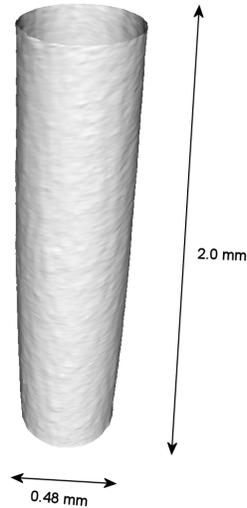
FIGURE 4: Hole measurement using FVM.
