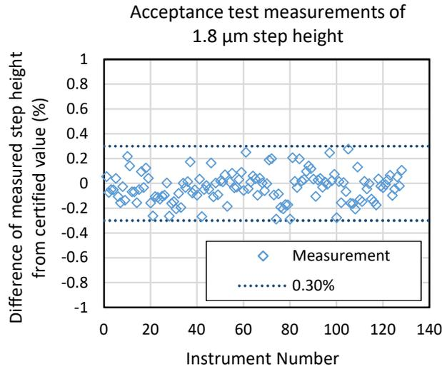
Figure 6: Measurements of 1.8  $\mu\text{m}$  step-height specimens on 130 interference microscopes, each one of which was independently calibrated using the wavelength method prior to acceptance testing in manufacturing. The relative standard deviation is 0.12% RMS.
