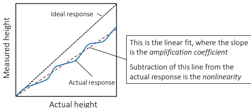
Figure 1: Height response of an instrument designed for determining surface heights.
