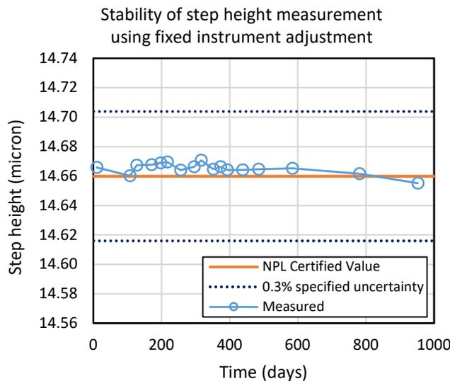
Figure 5: Measured height value for a certified step-height specimen, using a fixed adjustment value for the instrument over 960 days. The RMS stability is 0.04% without recalibration.
