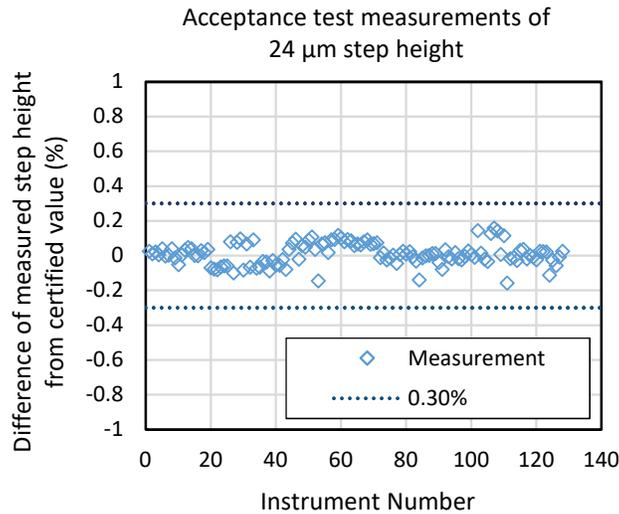
Figure 7: Measurements of 24  $\mu\text{m}$  step-height specimens on 130 interference microscopes, each one of which was independently calibrated using the wavelength method prior to acceptance testing in manufacturing. The relative standard deviation is 0.06% RMS.
