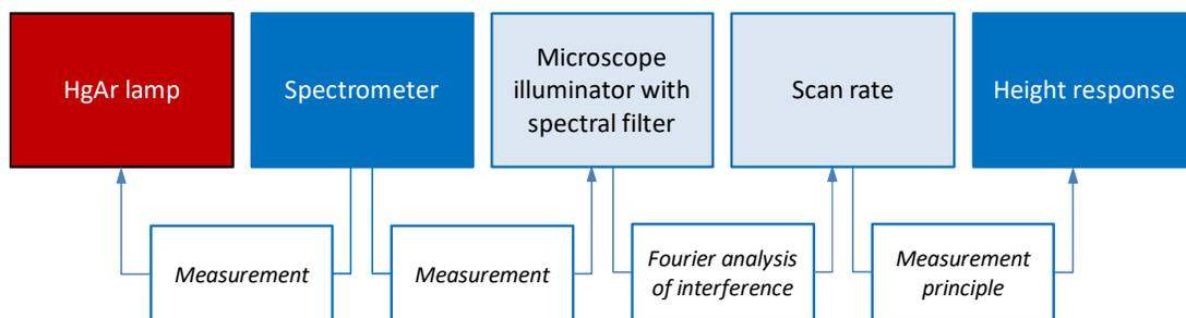
Figure 3: Traceability chain for calibration of the height response amplification coefficient of a CSI microscope using the wavelength method.
