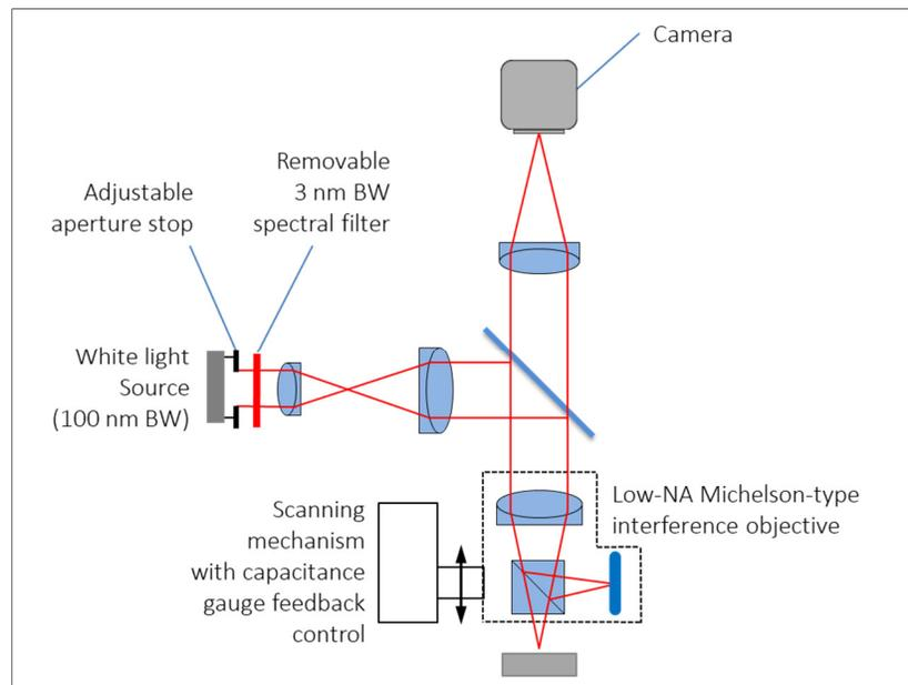
Figure 2: System layout of a Zygo coherence scanning interference microscope configured with a narrowband spectral filter and a low numerical aperture to calibrate the scanning mechanism as a transfer standard for traceable calibration of the amplification coefficient.
