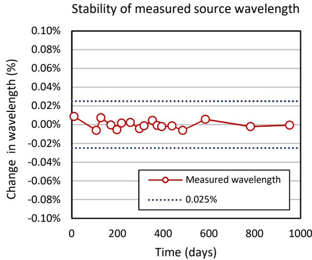
Figure 4: Measured mean wavelength of the spectrally-filtered microscope source illumination. The average value is 550.618 nm and the RMS stability is 0.005% over 960 days.
