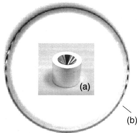
**Fig. 2** (a) 5-mm-diam diamond-turned cone with a 90-deg included angle. (b) Experimental image of the cone in the proposed spherical geometry showing an intersection ring with interference fringes.
