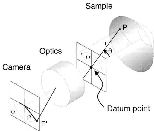
**Fig. 4** Mapping of the spherical measurement geometry to the imaging plane of the camera.
