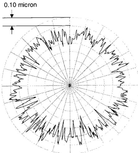
**Fig. 8** Circular slice through the data given in Fig. 6, showing the roundness profile.
