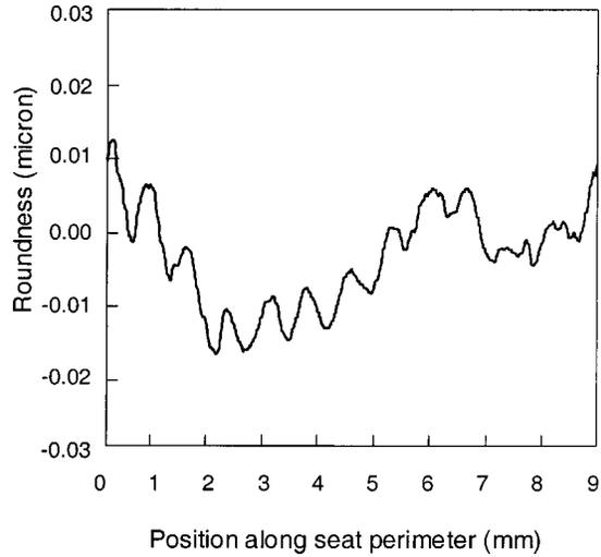
**Fig. 9** Alternative roundness display, this time of a diamond-turned surface.
