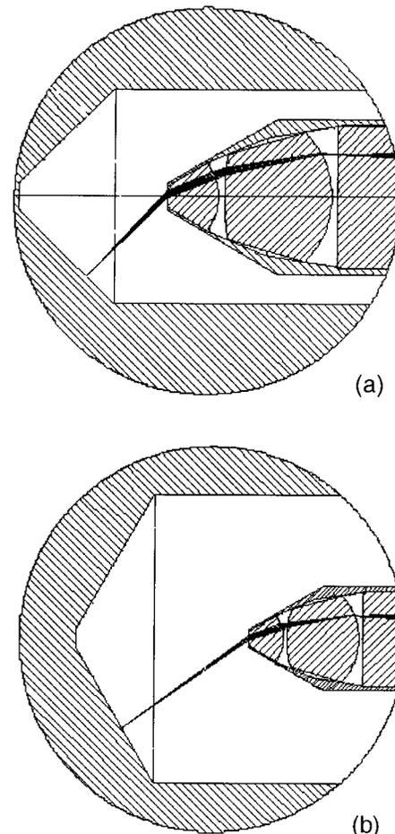
**Fig. 3** (a) Measurement probe cross section with a 90-deg included angle cone in a 4-mm-diam bore. (b) Same measurement probe but with a 120-deg included angle cone in an 8-mm-diam bore.
