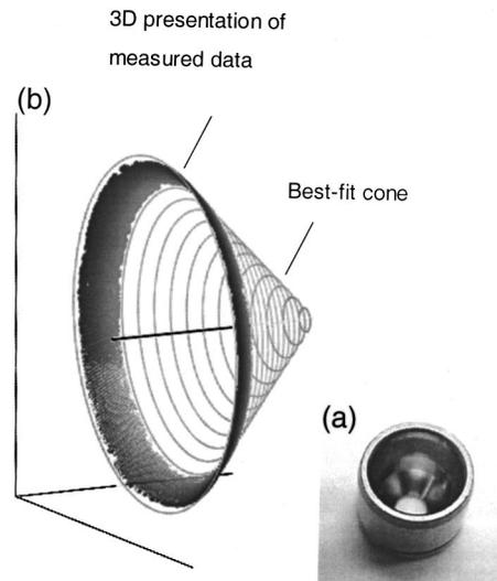
**Fig. 5** (a) Sample similar to an actual valve cone. (b) Experimental data and best-fit cone.
