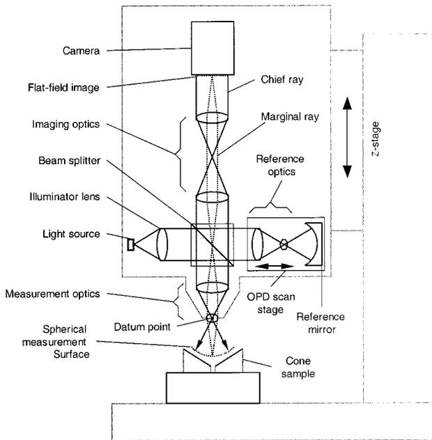
**Fig. 1** Conceptual design of the proposed optical gage for measuring valve cones.
