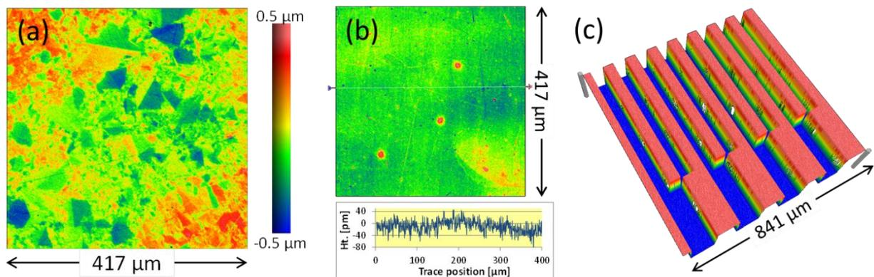
Fig. 3. Hybrid CSI/PSI results: (a) grains of SiC ‘flat’ measured using a 20X Mirau (NA = 0.4); (b) roughness of super-smooth optic, also measured with 20X Mirau; and (c) discontinuous 1.8- $\mu\text{m}$  steps measured using a 5X Michelson (NA = 0.13).
