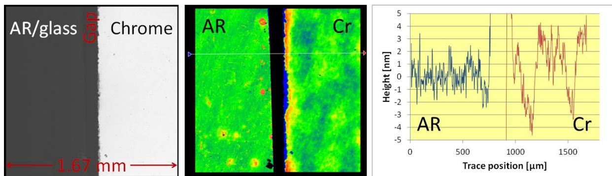
Fig. 2. Measurement of adjacent AR and chrome. *Left*: intensity image at non-saturating light level; *middle*: height map from HDR measurement; *right*: horizontal trace through AR and chrome.
