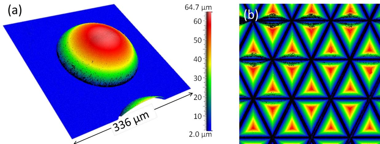
Fig. 1. Measurements of (a) polymer micro-lens using 3X DNR; and (b) retroreflector array using 4X DNR.
