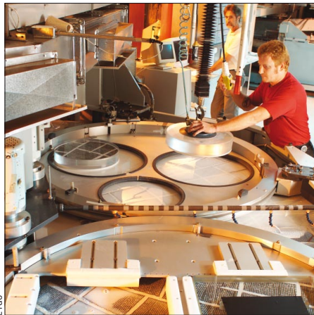
The AHMD (top) uses multiple off-axis optical paths. ZYGO manufactures high-precision metre-scale optics (bottom left) for customers including the National Ignition Facility.
