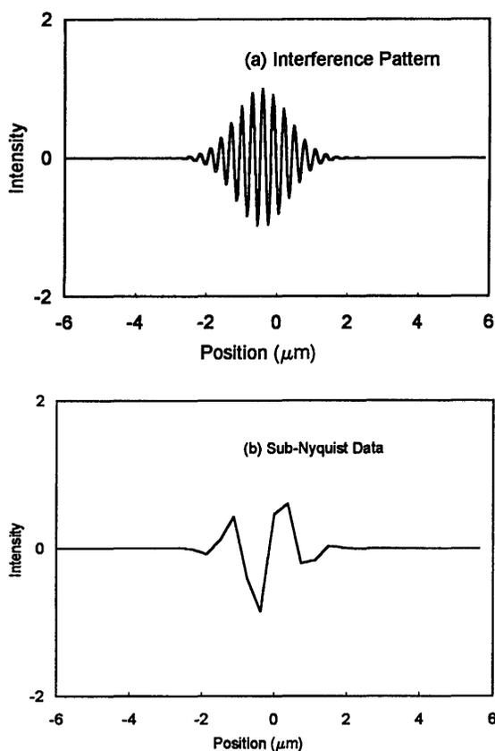
Fig. 2. Simulated interference data. (a) Dense sampling correctly represents the complete interference pattern. (b) Sub-Nyquist sampling (1 point every  $5\pi/2$ ) results in a severely distorted data set that is still useful for three-dimensional imaging if correctly processed.
