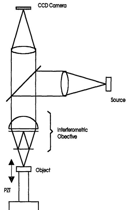
Fig. 1. Scanning white-light interferometer. The PZT translates the object in a direction perpendicular to the optical axis of the objective while intensity images are recorded with the detector array. These images are processed in the spatial frequency domain to generate a three-dimensional representation of the surface topography.
