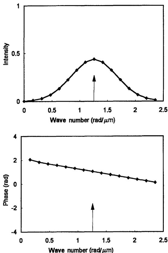
Fig. 3. Fourier transform of the sub-Nyquist data shown in Fig. 2(b). The arrow indicates the mean or peak wave number, which is much smaller than the actual mean wave number of the interference pattern because of undersampling. The phase information in (b) is used to calculate local surface height.
