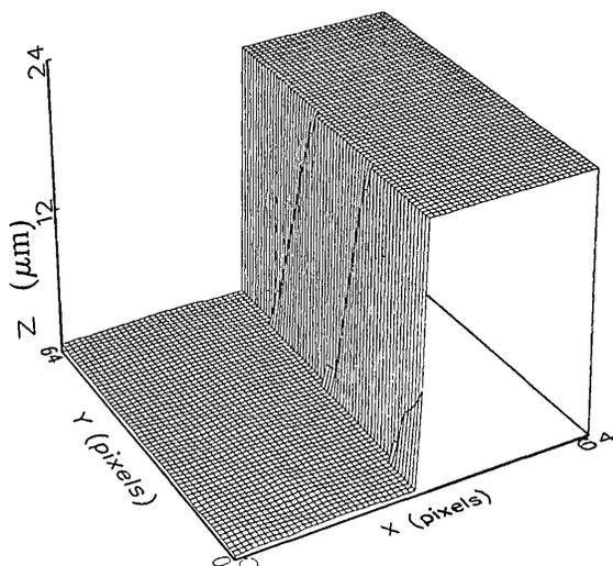
Fig. 4. Three-dimensional profile of a 20- $\mu\text{m}$  standard step height obtained from sub-Nyquist white-light interferograms. The repeatability of the measurement is 10 nm.
