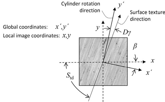
Figure 3. Determining lead angle from a local topography map.
