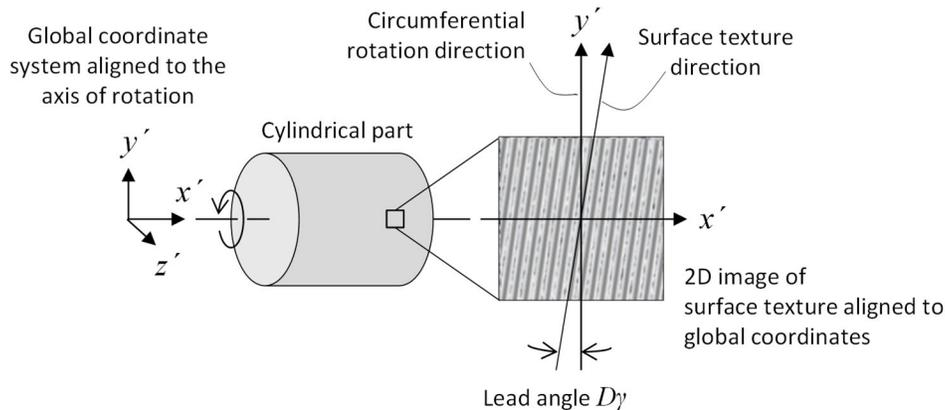
Figure 2. Geometrical definition of the machining lead angle for a cylindrical part.
