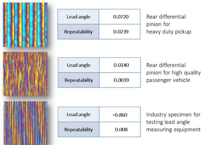
Figure 5: Examples of surface texture and measured lead angle for three different surface textures.
