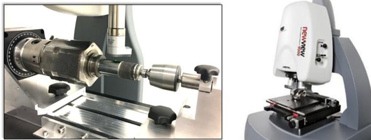
Figure 4: Left: Staging for a sample part. Right: Interference microscope for measuring areal surface topography.
