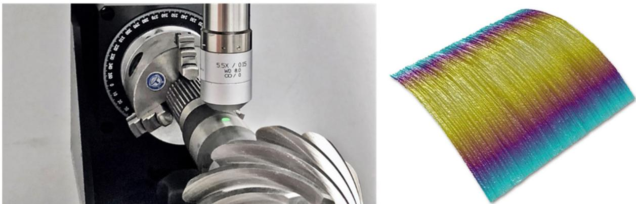
Figure 1. Experimental geometry (left) and example topography (right) for a shaft measurement.
