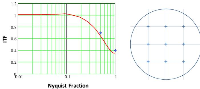
Figure 3: Measured system ITF (red line) as determined with a step artifact at the 9 field locations indicated on right. Each field location produced the same ITF. The blue diamonds represent the design goals for the half and full Nyquist frequencies.
