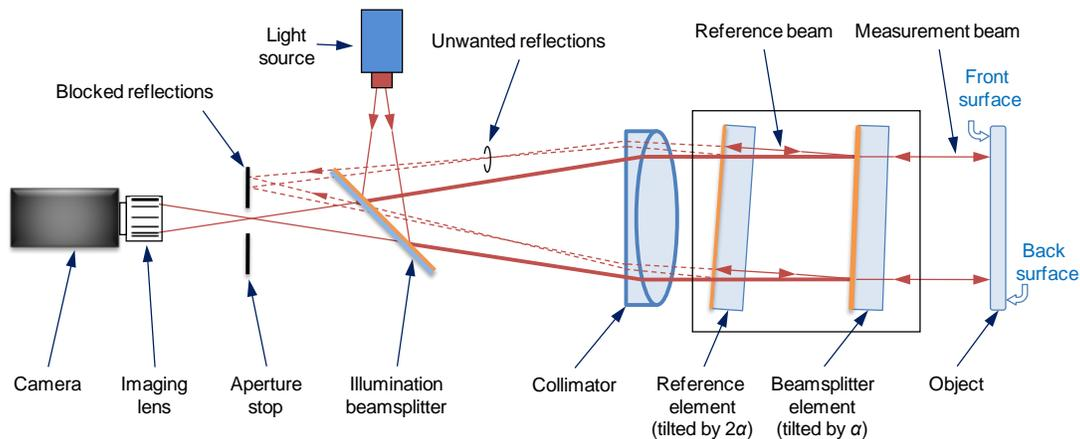
Figure 1: Basic optical layout. A broad-band extended source illuminates an interferometer cavity consisting of the 1<sup>st</sup> surfaces of the reference and beam-splitter elements and the object. The object surface is set to the equal-path location and focused onto the camera. Phase shifting is accomplished by moving the boxed elements as a whole.
