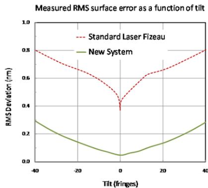
Figure 4: RMS residuals as a function of part tilt for the FGT compared to a standard laser Fizeau. The measurements have been high pass filtered with a 1mm cutoff to minimize turbulence affects.
