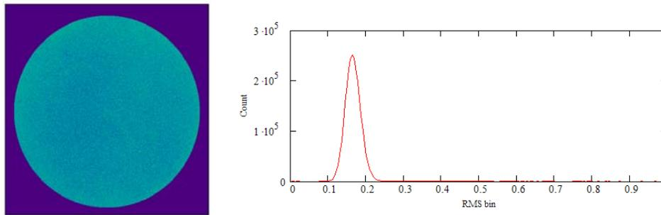
Figure 2: The uncertainty matrix calculated from an ensemble of 40 measurements.
