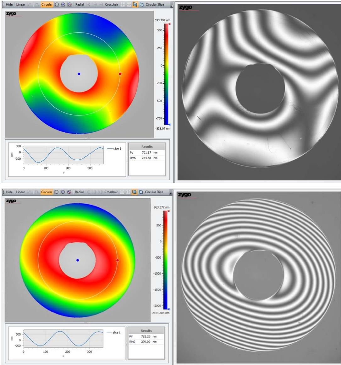
Figure 5: Measurements of 65mm hard disk blanks made of aluminum (top) and glass (bottom).
