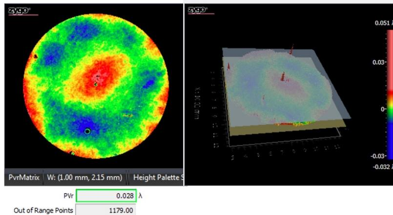
Figure 2. Pvr of the same part. Note that it easily meets the specification and only 1179 of 380,000 points (0.3%) were removed.
