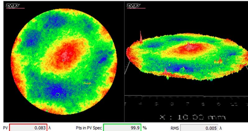
Figure 1. Test part with  $0.05 \lambda$  specification. Small spikes in data cause it to fail but only 0.1% of the surface is out of spec so a Points in PV Specification tolerance of 99% would allow this part to pass.
