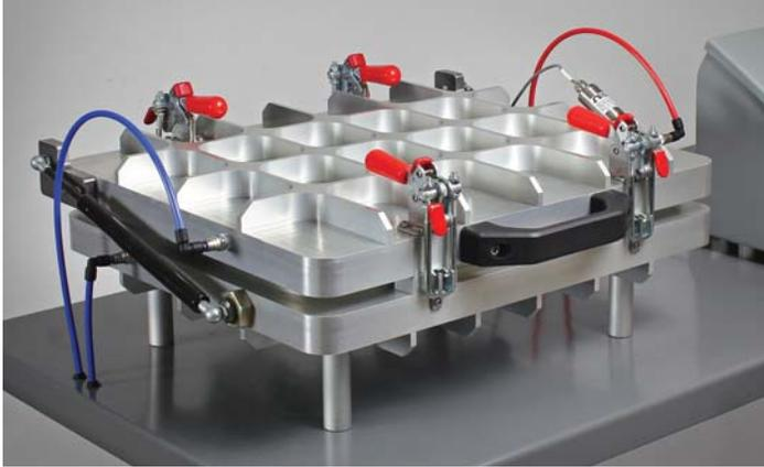
Figure 3: ZYGO custom-designed proof pressure test fixture
