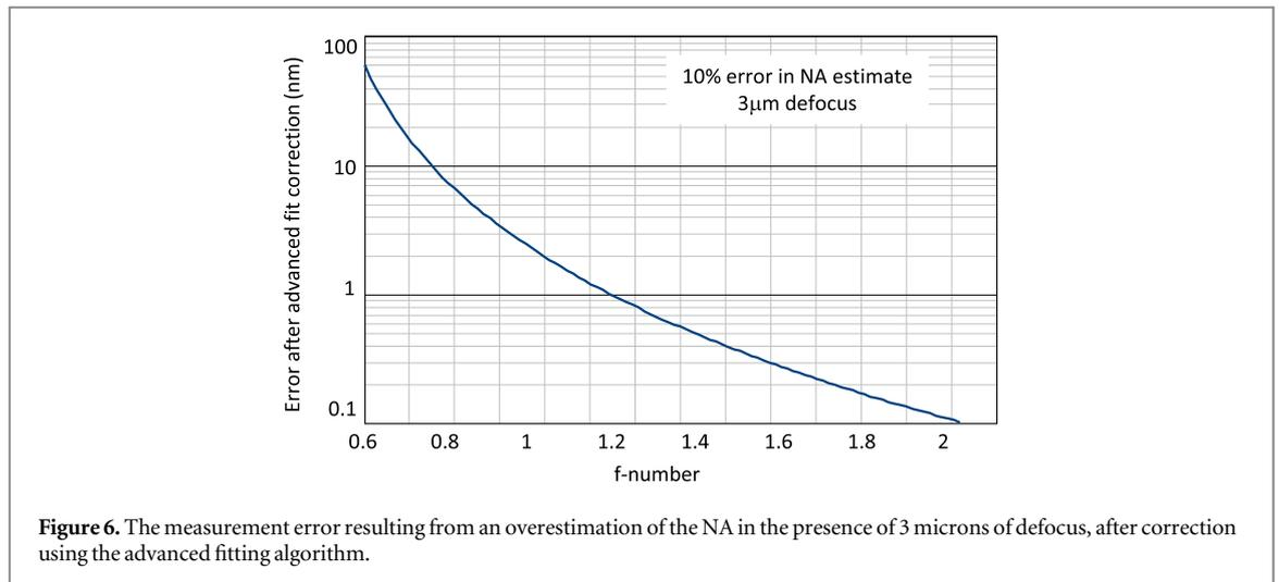
**Figure 6.** The measurement error resulting from an overestimation of the NA in the presence of 3 microns of defocus, after correction using the advanced fitting algorithm.
