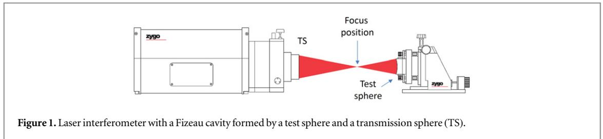
**Figure 1.** Laser interferometer with a Fizeau cavity formed by a test sphere and a transmission sphere (TS).
