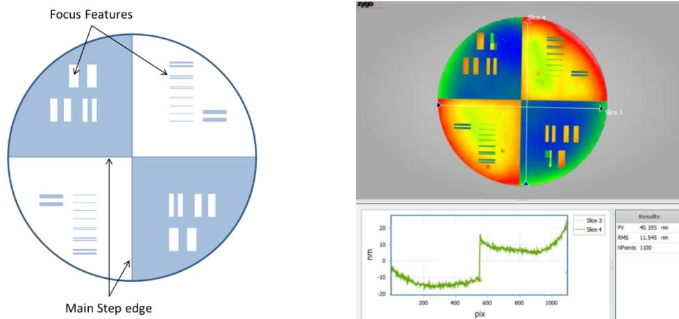
Figure 1: Left—ITF test sample design. Right—Measurement result.
