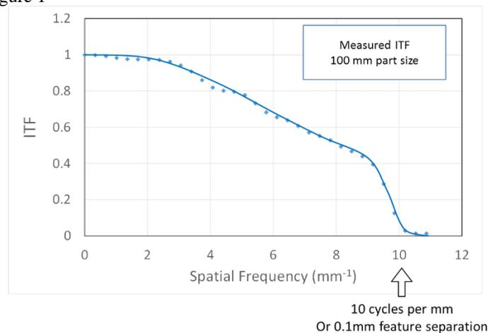
Figure 2: Example precision ITF measurement results showing a design resolution limit of 1000 cycles over a 100mm aperture.
