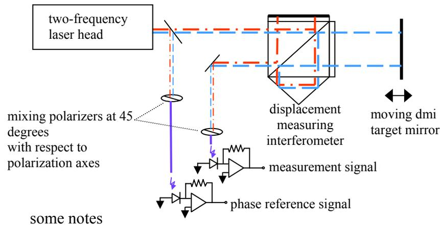
Figure 1 – Ideal heterodyne displacement measuring interferometer system minus phase interpolator
