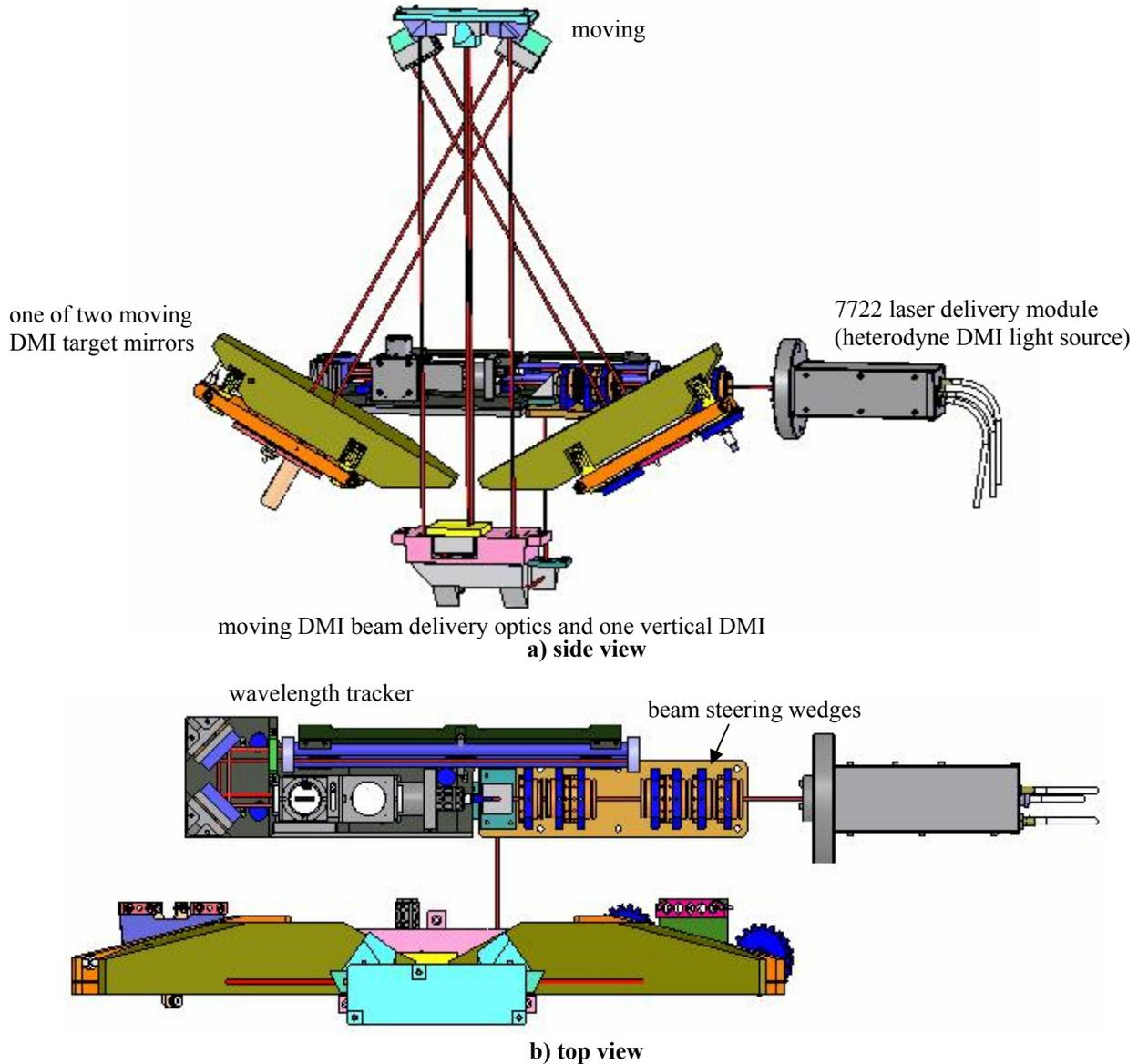
**Figure 2 – 4-axis DMI system<sup>3,4,5</sup>**
