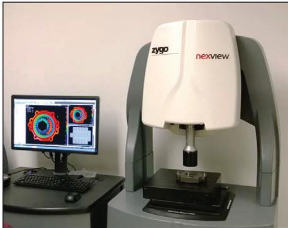
**FIGURE 2.** Multi-functional interference microscope system with interchangeable objectives, here configured with the 0.5X objective.
