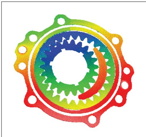
FIGURE 9. 3D image of the part shown in the previous figure.  $Sq = 26.7\mu m$ ,  $Sz = 119.8\mu m$ .
