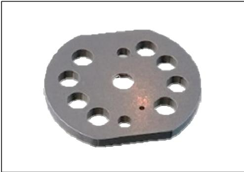
FIGURE 4. Photograph of a 29-mm diameter machined fuel injector component.
