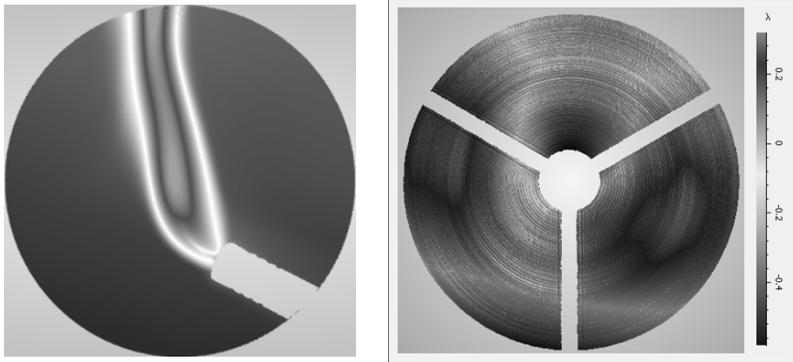
Figure 4: Dynamic measurements using single-camera frame laser interferometry. Left: an air-density profile within a candle flame. Right: Surface of diamond turned part having a 500nm of surface departure. The field of view is 100mm.
