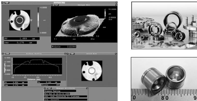
Figure 2: Surface profiling of automotive parts using white light interferometry.
