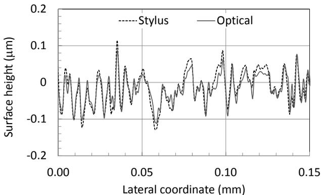
Figure 3: Comparison of cross-sectional profiles obtained with an optical profilometer and with a mechanical stylus tool.[5]
