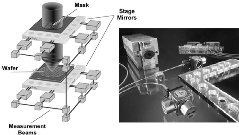
Figure 1: Interferometric stage control—a traditional example of optical metrology in the service of precision engineering.
