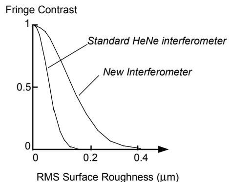
**Figure 1.** Improvement in fringe contrast with the  $1.55\mu\text{m}$  interferometer.
