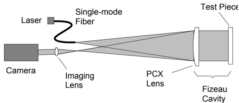
**Figure 4.** Near-infrared laser diode interferometer for flat surface testing.
