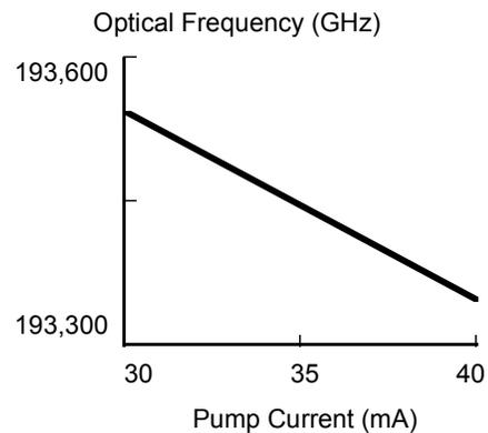
**Figure 5.** Tunability of laser diodes.
