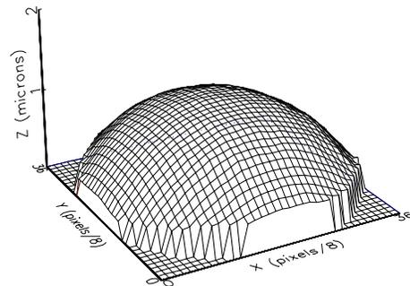
**Figure 3.** Height map for a 75-mm diameter ground glass surface ( $5\text{-}\mu\text{m}$  grit).
