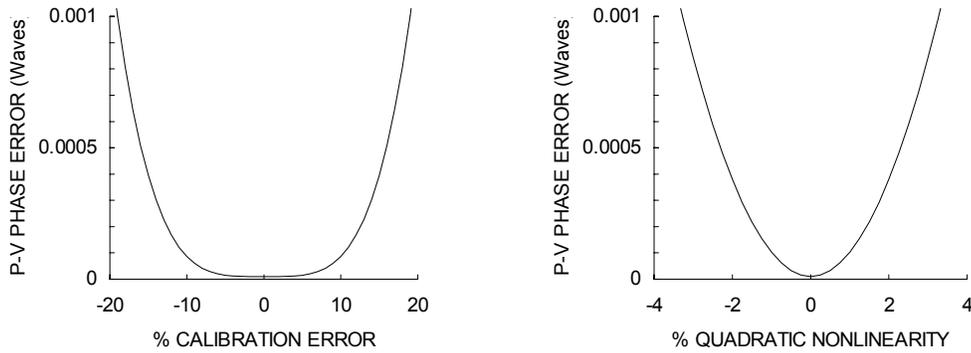
**Figure 6.** Performance of interferometer in the presence of first- and second-order distortions in the phase shift (left and right, respectively). The high accuracy of the laser diode interferometer is due in part to the relative insensitivity of the seven-frame measurement procedure to distorted phase shifts.
