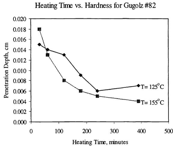
Therefore, if during manufacturing or packaging, the pitch is heated for different time periods, or at different temperatures, the properties of the pitch could dramatically change. Furthermore, once in the optics shop, if the melting procedures are not well controlled to maintain a consistent melt time and temperature, one can expect variation in the performance of each new lap poured.
