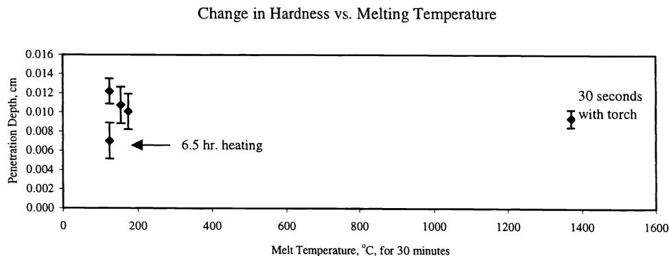
To gain more insight into the effect of melting time on pitch hardness, several samples were prepared at 125°C and 155°C and melted between 30 to 400 minutes. The penetration depths of the resulting samples are plotted in Figure 3. For both temperature ranges, the pitch hardness doubles for longer melting times. It also appears that the pitch hardness stabilizes
