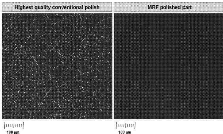
**Figure 4: After etching, comparison of dark-field microscopy on highest quality, conventionally polished parts and MRF polished parts illustrate the dramatic decrease in scatter sites and “chatter marks” normally associated with subsurface damage from conventional finishing.**
