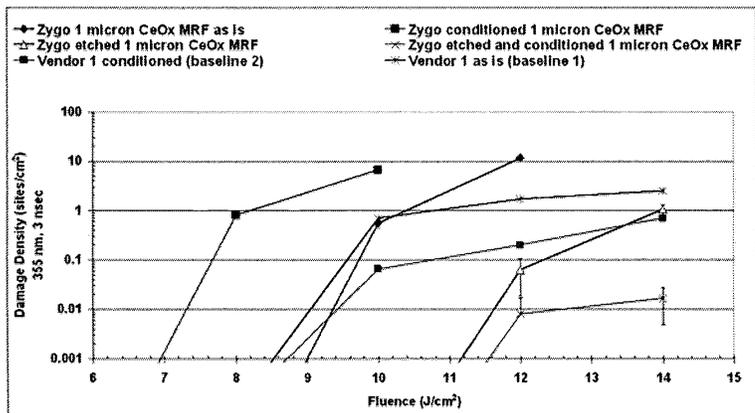
**Figure 3: Damage density observed at 355 nm, 3 nsec, on 15.2 cm diameter by 1.0 cm thick fused silica samples polished by Zygo using ZrOx conventional polishing techniques and final polished using MRF to remove 1 μm of material.**
