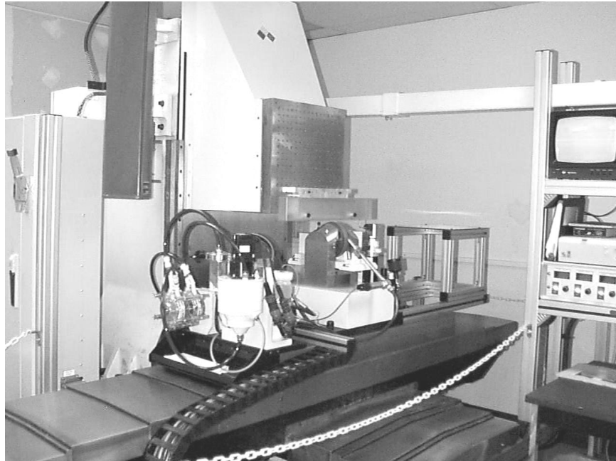
Figure 1. 150-mm wheel raster MRF machine (side view)
