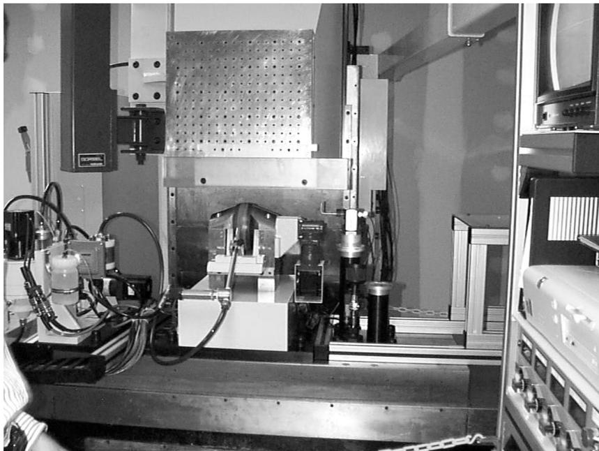
Figure 2. 150-mm wheel raster MRF machine (front view)
