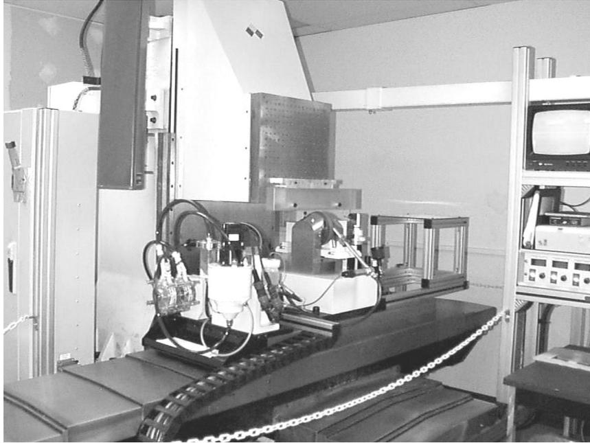
Figure 1. 150-mm wheel raster MRF machine (side view)
