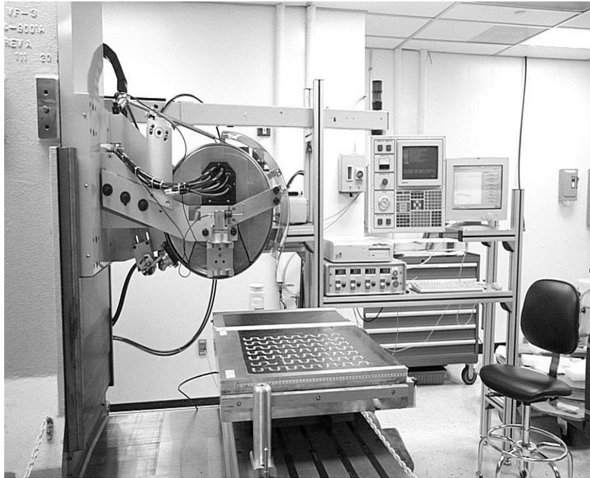
Figure 3. 500-mm wheel raster MRF machine (side view)
