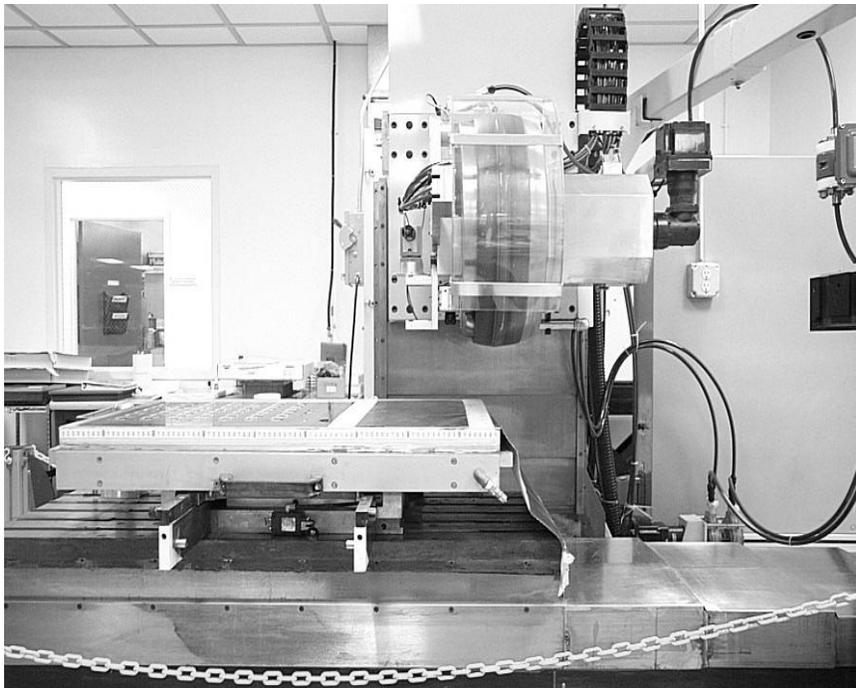
Figure 4. 500-mm wheel raster MRF machine (front view)
