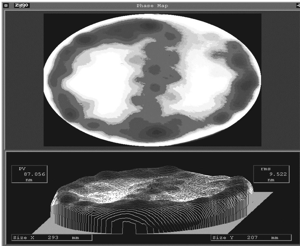
Figure 7. Mirror surface figure after conventional polishing
