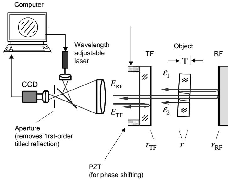
**Figure 2:** Schematic of transmitted wavefront geometry showing spurious reflected electric fields  $\epsilon_1, \epsilon_2$  and the addition of a wavelength-adjustable laser source.
