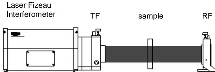
**Figure 1:** Familiar transmitted wavefront test geometry using a commercial laser Fizeau interferometer.
