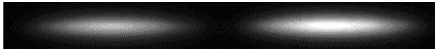
Figure 7: Fluorescence image recorded for a 20- \mu\text{m} fiber core, in the case of a large beam shear. The difference in intensity is due to a vertical misalignment of one beam.
