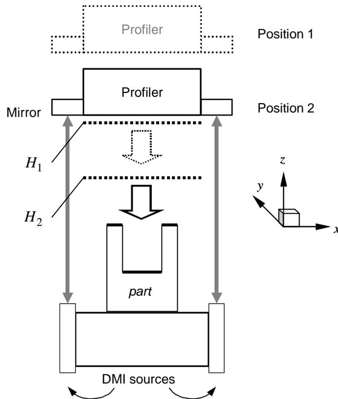
**Figure 2:** Basic measurement geometry for step height measurements using IR coherence scanning profilometry combined with displacement measuring interferometry.
