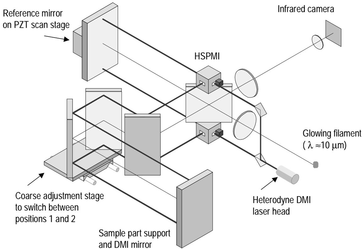
**Figure 3:** Example geometry for a step-height measurement system based on infrared scanning interferometry combined with a two-axis laser displacement gage and two high-stability plane mirror interferometers (HSPMI).
