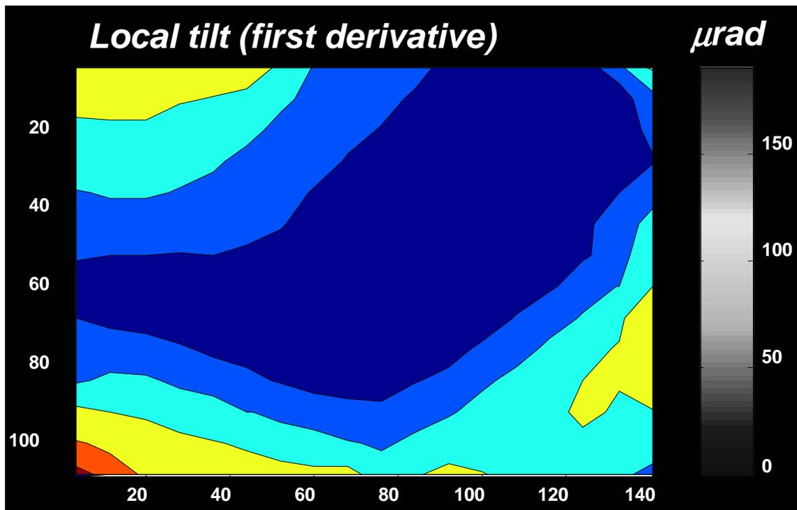
Figure 8: Local tilt (slope) in micro-radians of an 800 $\mu$ m hard pellicle mounted on a 157nm clear blank reticle.
