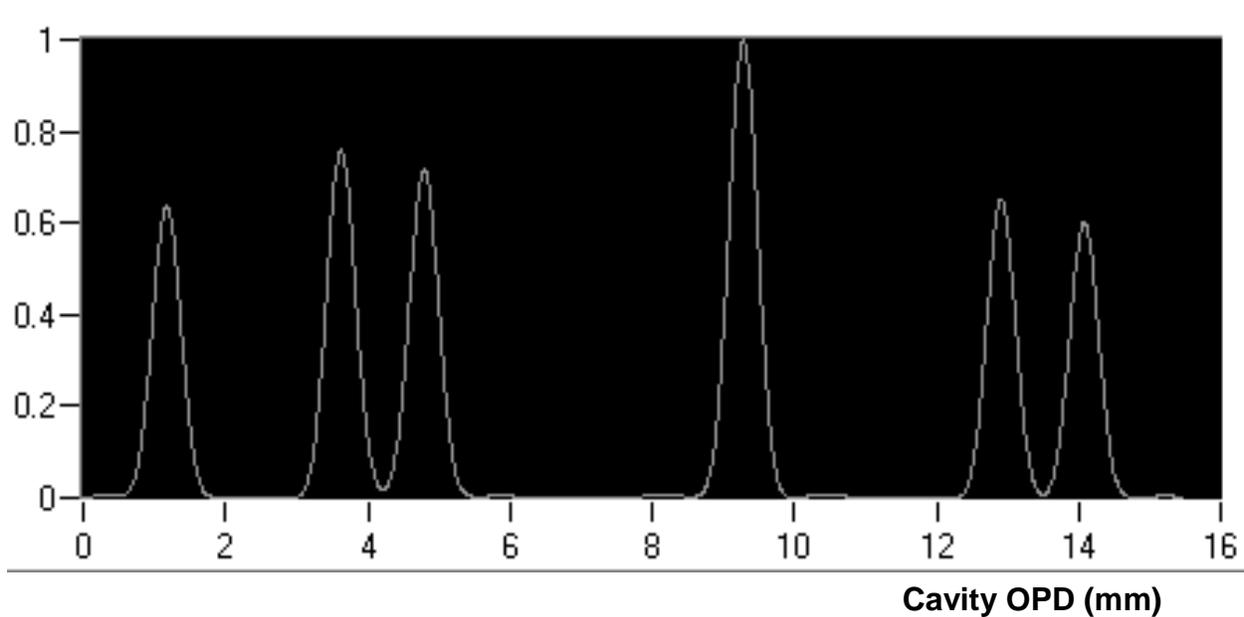
Figure 4: The optical path distance spectrum for an 800μm hard pellicle mounted on a 157nm reticle blank. From left to right, the six peak positions correspond to the optical path distances: (1) pellicle optical thickness; (2) pellicle back to reticle front; (3) pellicle front to reticle front; (4) reticle optical thickness; (5) pellicle back to reticle back; and (6) pellicle front to reticle back.
