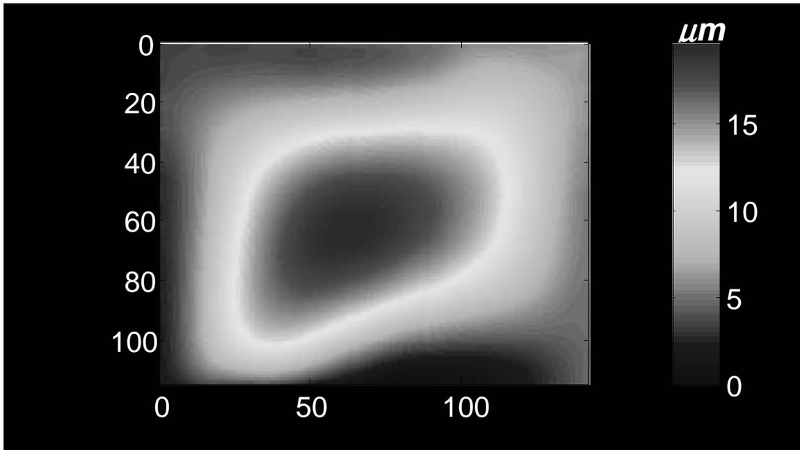
Figure 9: Reticle-pellicle gap variation in microns between a 300 $\mu\text{m}$  hard pellicle mounted on a chromed blank reticle. The global tilt has been removed. The measured sag of  $\sim 19\mu\text{m}$  in the pellicle center matches closely to the  $16\mu\text{m}$  predicted sag due to gravity.
