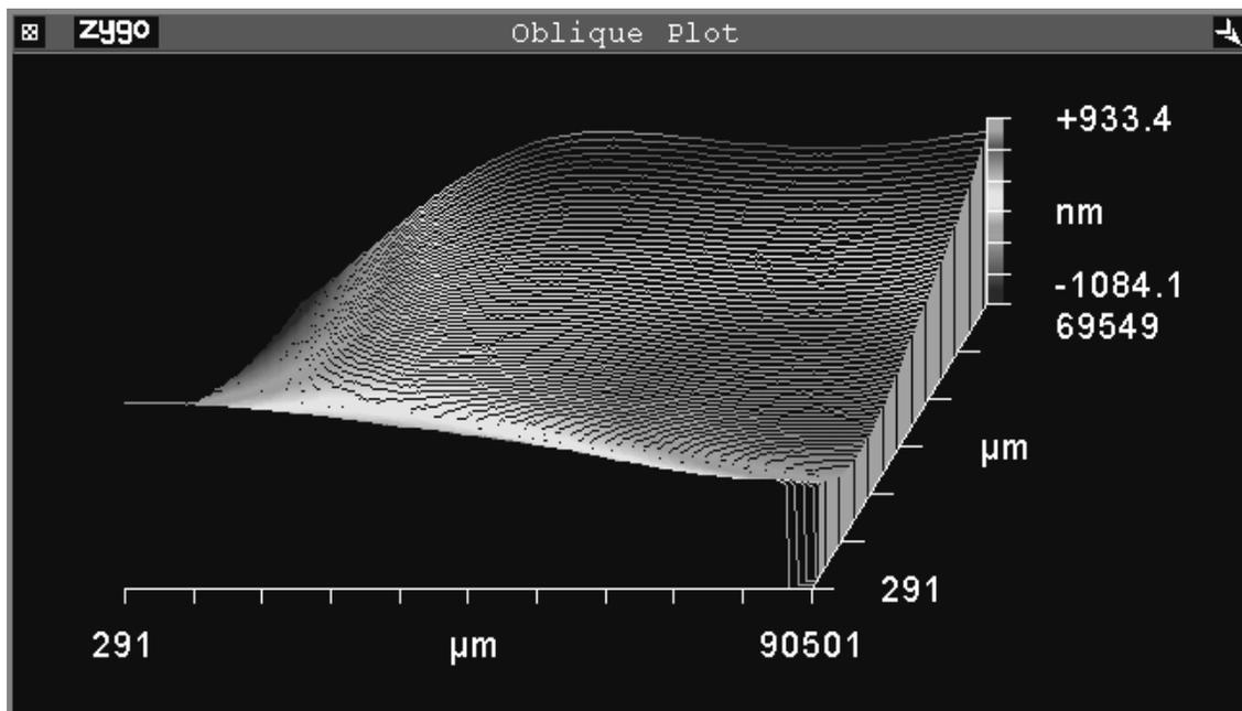
Figure 7: Measured variation of the pellicle to reticle gap with the 42  $\mu$ radian wedge removed.
