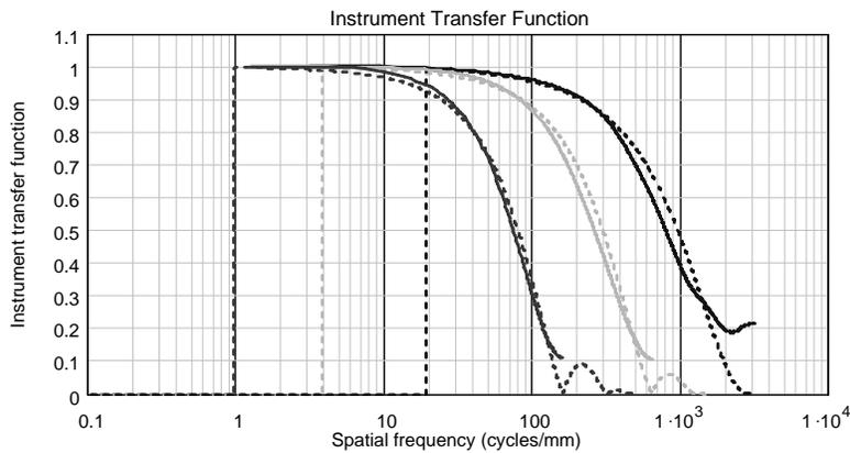
Figure 8: Comparison between measured (solid) and theoretical (dashed) results for the (left to right) 5X, 20X and 100X interferometric microscope objectives demonstrates good agreement when using a step height artifact to evaluate ITF.
