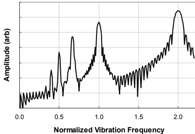
Figure 1: Phase error sensitivity of a PSI algorithm as a function of vibrational frequency normalized to the sample rate
