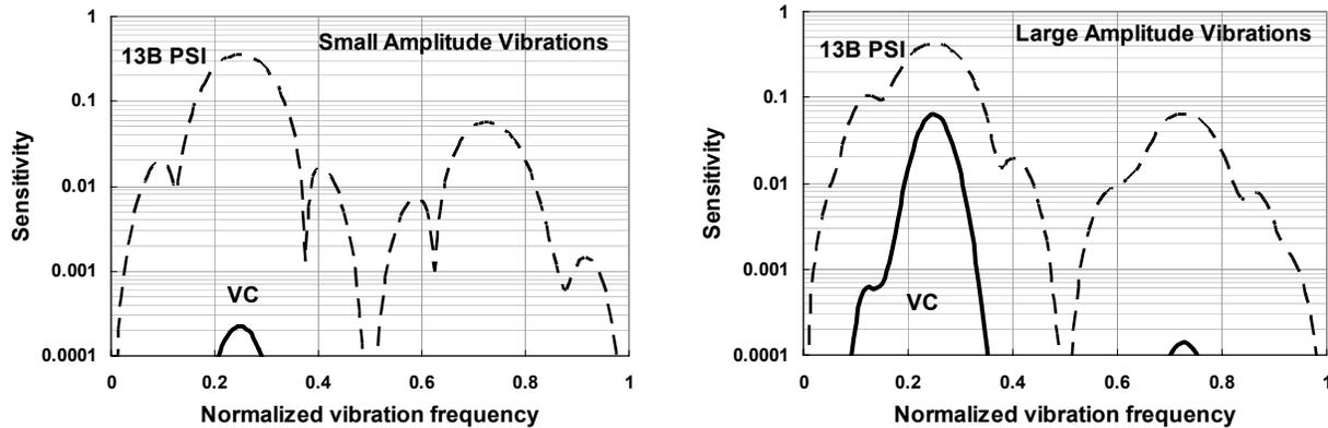
Figure 4: Phase error sensitivity for the 13-frame algorithm (dashed line) and VC (solid line) for small amplitude (5nm) and large amplitude (50nm) vibrations.
