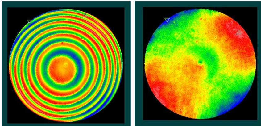
Figure 3: Measurement of a spherical part with  $\sim 3$  fringes of departure disturbed with a 25nm amplitude vibration at a frequency of  $\frac{1}{4}$  of the frame rate before (left) and after (right) processing with the VC algorithm. The 20nm PV ripple observed in the original profile was reduced by  $>25X$ .
