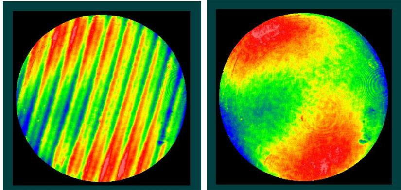
Figure 2: Measurement of a flat part with  $\sim 5$  fringes of tilt disturbed with a 15nm amplitude vibration at a frequency of  $\frac{1}{4}$  of the frame rate before (left) and after (right) processing with the VC algorithm. The 15nm PV ripple observed in the original profile was reduced by  $>25X$ .
