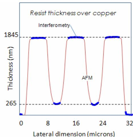
Figure 7: Comparison of interferometry with AFM measurements of the thickness of patterned photoresist. The AFM result derives from a top-surface measurement relative to the surrounding uncoated area. Correlation is <10nm.
