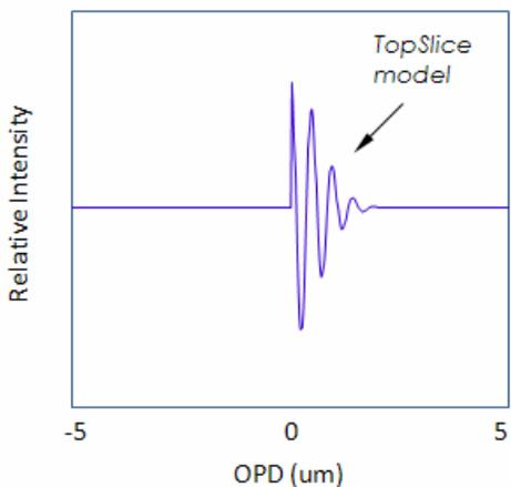
Figure 4: Creating a TopSlice model signal from the original opaque-surface SWLI signal in Figure 2.
