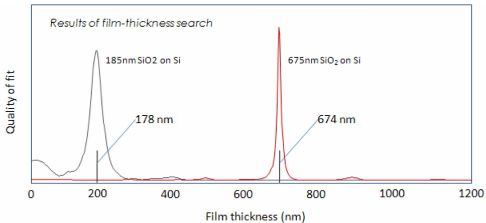
Figure 9: Results of a search through a range of 0-1200nm film thicknesses to find a match of theoretical to experimental signals for two different SiO<sub>2</sub> on Si film thickness standards: 185nm and 675nm. The vertical axis quantifies the quality of fit, with higher values corresponding to a better frequency-domain match of theory to experiment.
