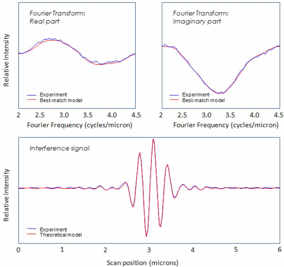
Figure 8: Frequency-domain (Top 2 graphs) and time-domain (lower graph) representations of a SWLI signal from a 185-nm SiO<sub>2</sub> film on Si, comparing the experimental signal with the best-fit from the model signal library.
