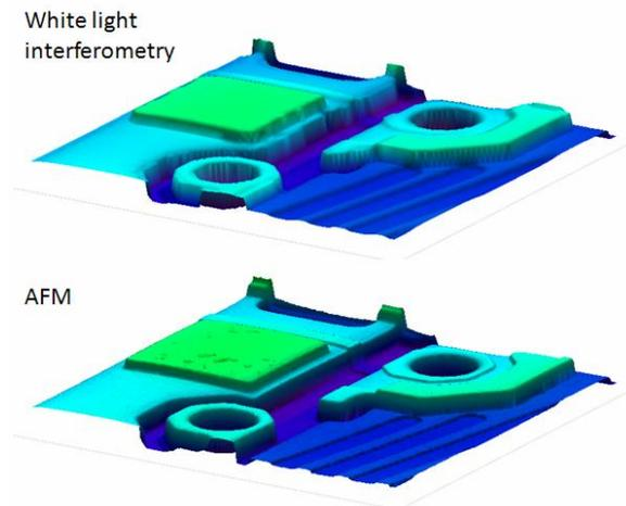
Figure 6: Comparison of interferometry with AFM measurements of the top surface of a thin-film transistor. The images are 40 microns square.
