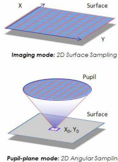
Figure 10: Concept illustration of the transition from SWLI imaging mode to pupil-plane mode.
