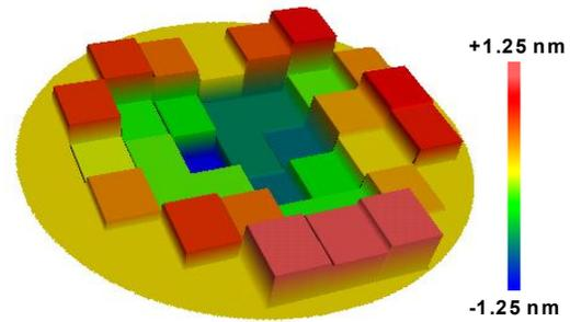
Figure 13: Variation in thickness of a nominally 80-nm thick Si<sub>3</sub>N<sub>4</sub> film on a silicon wafer by measurement site, using the pupil-plane technique.
