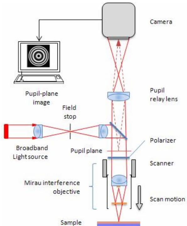
Figure 11: Scanning white light interferometer in pupil-plane mode for detailed film structure analysis.
