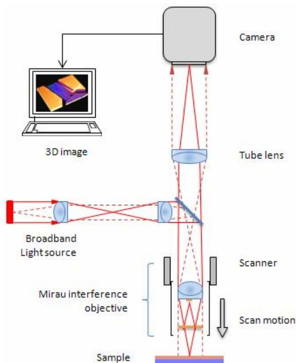
Figure 1: Scanning white light interferometer for 3D surface measurements. In this paper, all results are for a 0.8-NA objective, a 110-nm spectral bandwidth and 570-nm center wavelength.
