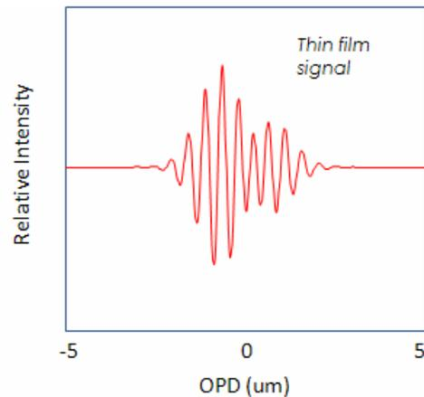
Figure 3: SWLI signal for a thin-film surface structure.
