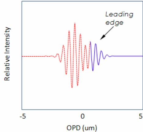
Figure 5: Locating the leading edge of the thin-film signal in Figure 3 using the TopSlice model signal with an adjustable amplitude and phase.
