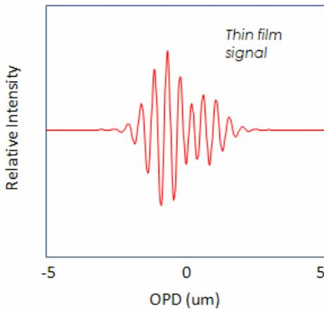
Figure 2: SWLI signal generate by the instrument shown in Figure 1
