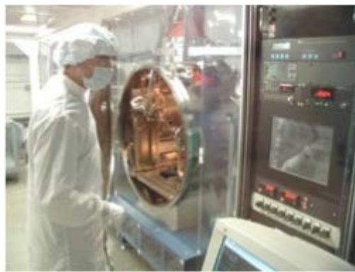
Figure 6. Ion Beam Figuring (IBF) chamber
