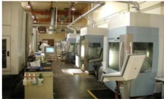
Figure 5. Five-Axis, Ultrasonic, High-Precision Milling Machines
