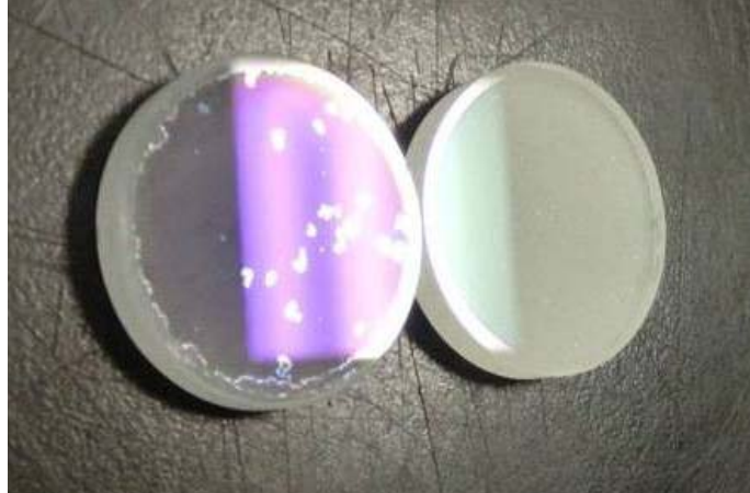
Figure 11. Witness samples of ZnS coatings, sample on left showing degradation after extreme environmental exposure and the sample on the right showing no degradation after extreme environmental exposure.
