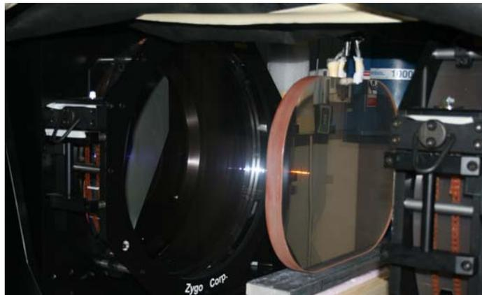
Figure 5. Cleartran™ window in a 24" Zygo MST Interferometer.
