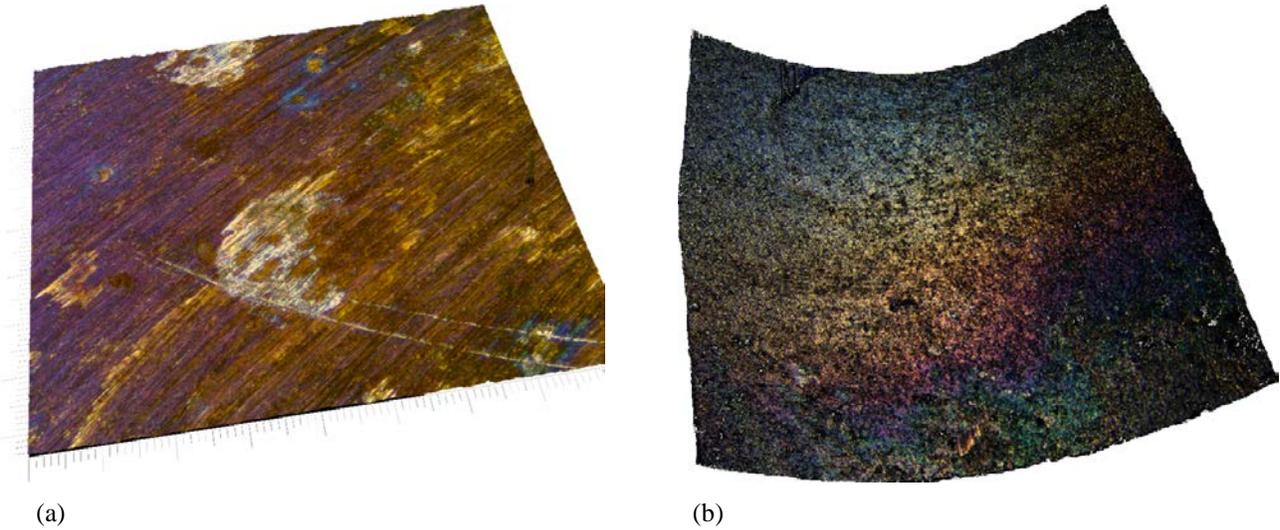
Figure 8. (a) 0.8 mm x 0.8 mm hybrid topography and color map showing local blemishes on a machined surface. (b) 1.7 mm x 1.7 mm hybrid map showing discoloration of a conical valve seat as a result of heat treatment.
