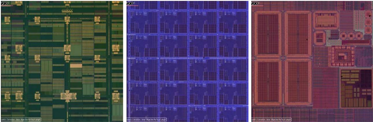
Figure 12. Examples of semiconductor wafers imaged in color as part of a CSI measurement. The field of view is 16.7 mm x 16.7 mm.
