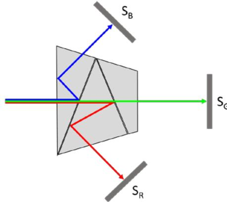
Figure 3. Principle of prism-based color channel separation for multi-detector color camera.
