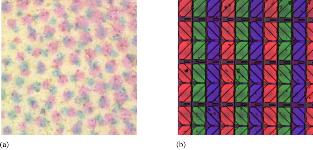
Figure 5. Intensity data captured by a CSI instrument for (a) ink pigments on high-gloss paper and (b) an array of color filters for flat panel displays. These images match those of Fig. 1.
