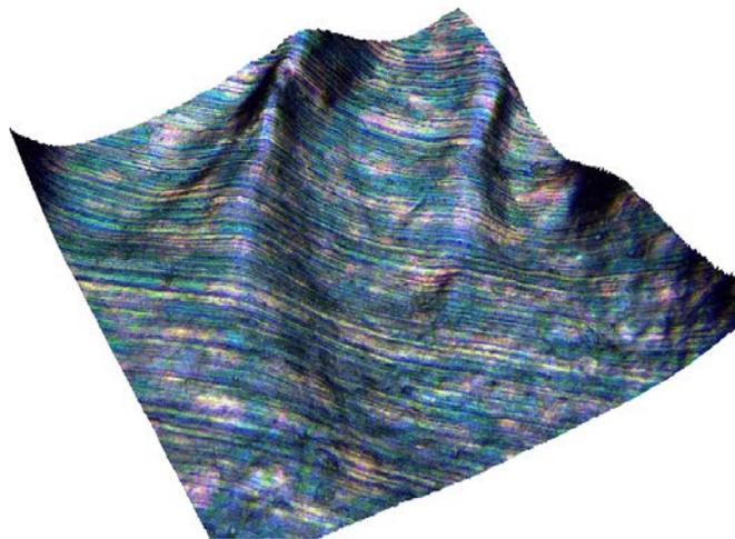
Figure 7. Hybrid map combining surface topography with measured color reflectivity for a piece of metallic wrapping paper. The field of view is about  $850\ \mu\text{m}$  on the side and the height range about  $32\ \mu\text{m}$ .
