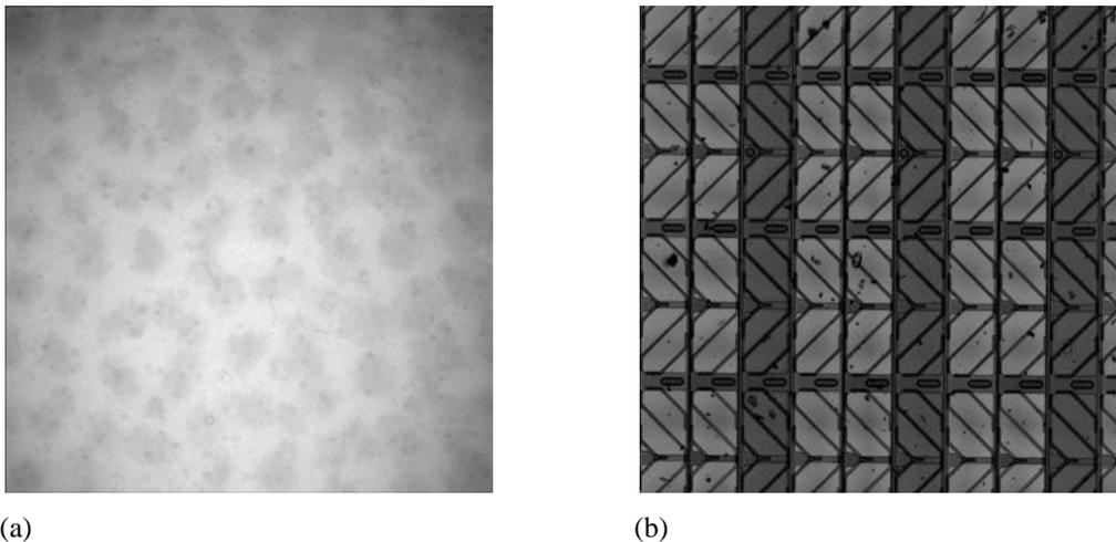
Figure 1. Intensity data captured by a CSI instrument for (a) ink pigments on high-gloss paper and (b) an array of color filters for flat panel displays.
