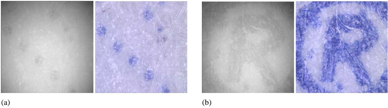
Figure 6. "Invisible" ink pigments on security paper. (a) shows monochrome and color data for ink dots that will appear in the scanned image of a bank note or check but are otherwise invisible to the unaided eye. (b) shows a "registered" symbol.
