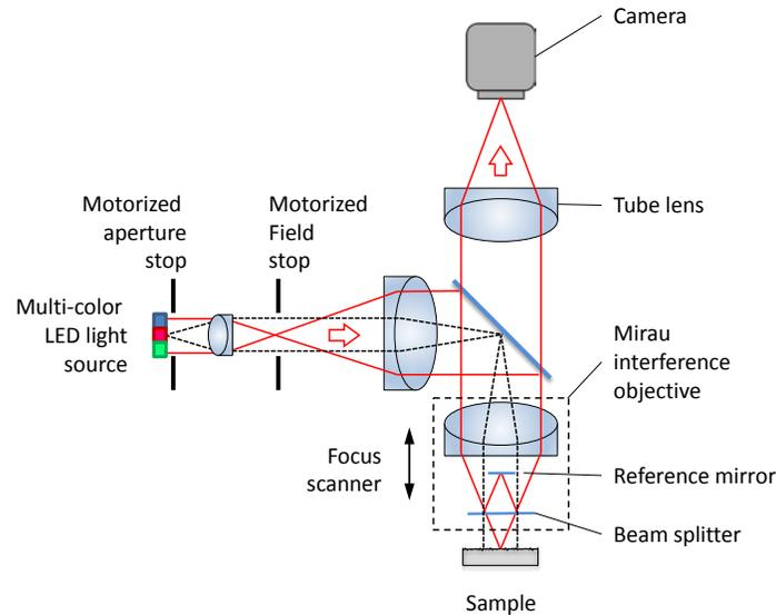
Figure 4. Simplified sketch of color-imaging CSI instrument, using a monochrome camera and a multi-LED illuminator.
