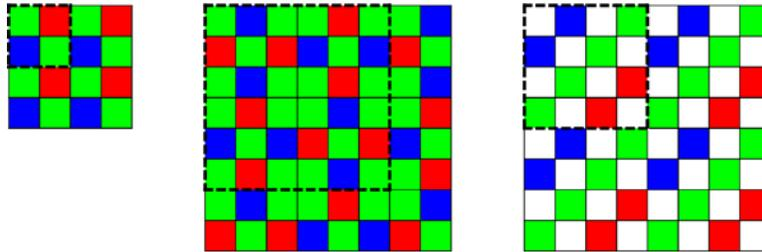
Figure 2. Example of 2x2, 6x6 and 4x4 color filter mosaics in use on color cameras. The dashed line delimits the elementary pattern.
