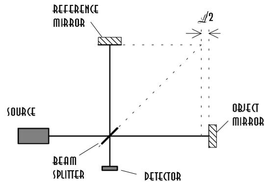
Figure 2: Michelson interferometer.
