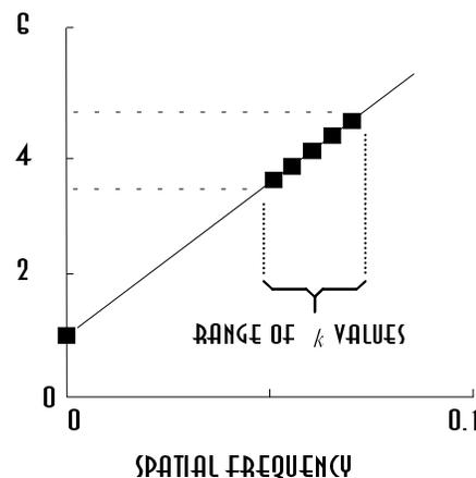
**Figure 6:** The *NewView 200* solves the ambiguity problem with white light, which provides phase information for a range of spatial frequencies  $k$ .
