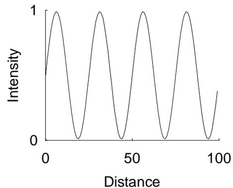
Figure 3: Variation of measured intensity with object distance in an interferometer.
