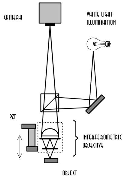
**Figure 7:** Optical system for scanning white light interferometry.
