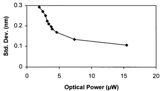
**Figure 10.** The measurement noise versus the optical power.
