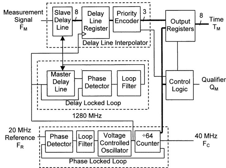
Figure 2. The block diagram of the phase meter.
