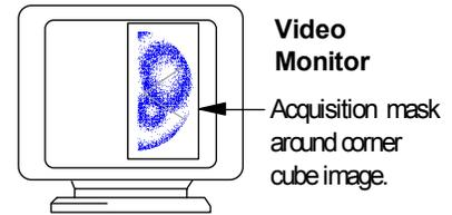
Use the Single Pass test when measuring very small or irregularly shaped prisms. Note that in the single pass test, any asymmetrical wavefront errors introduced by the interferometer are not canceled out as they are with the double pass test. In fact, any such wavefront errors will appear to be twice as severe as they really are and will affect the measurement results accordingly.
