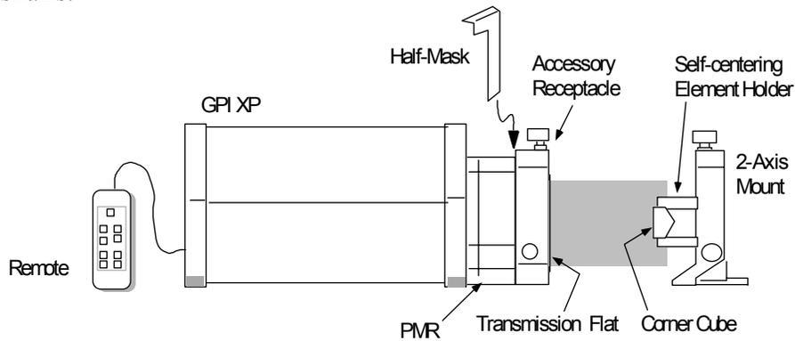
5. Mount the corner cube in the fixture, such that its face is parallel to the face of the Transmission Flat. Then position the corner cube in the measurement beam.
